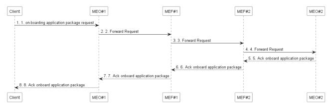
Figure 5.2.2.5.2-1: On-boarding application package in MEC federation
