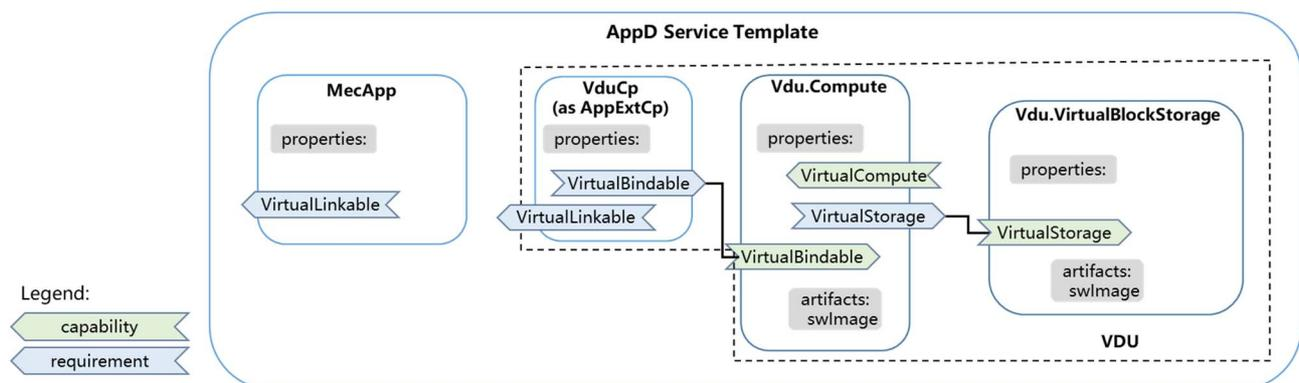
NOTE 1: The external connection points of the MEC app are represented using the VduCp node type according to the mechanism defined in clause A.3.2 of ETSI GS NFV-SOL 001 [3].
