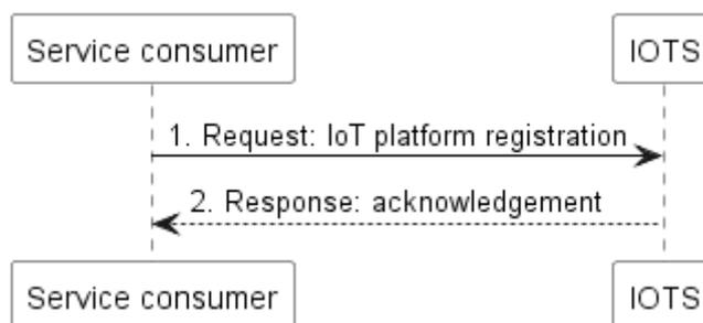
**Figure 5.3.4-1: Flow of IoT platform registration**
