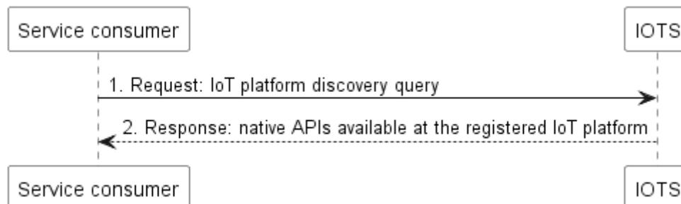
**Figure 5.3.3-1: Flow of IoT platform information request**
