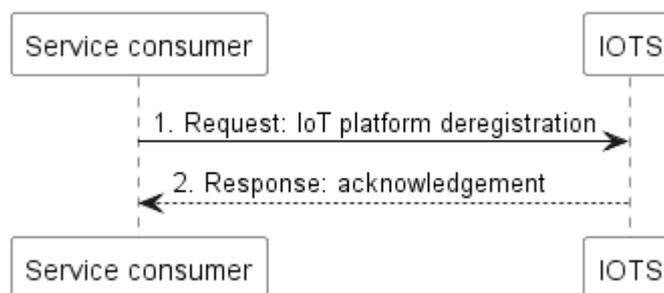
**Figure 5.3.6-1: Flow of IoT platform deregistration**
