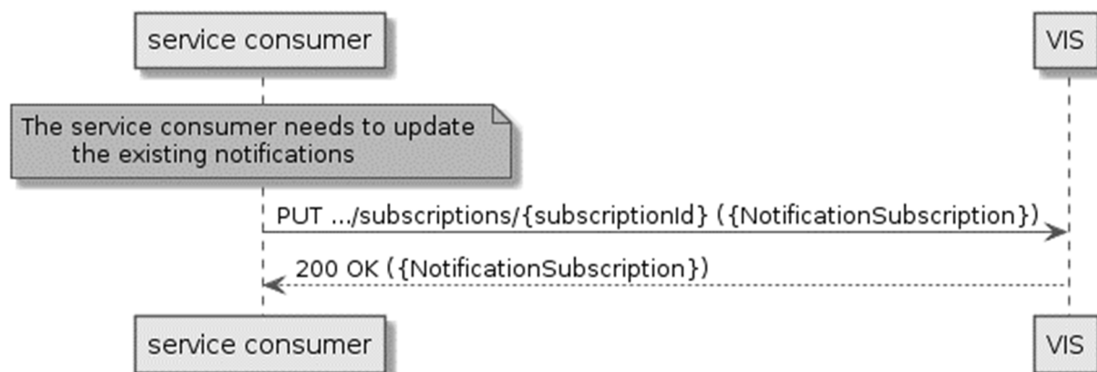
Figure 5.5.6.3-1: Flow of service consumer updating subscription for V2X information event notifications
