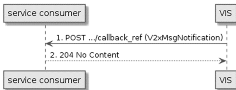
Figure 5.5.9.3-1: Flow of V2X message notification
