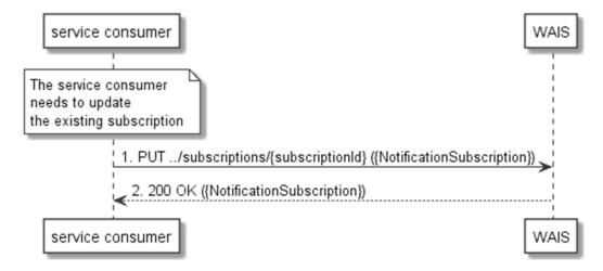
Figure 5.2.4.3-1: Flow of service consumer updating subscription for WLAN event notifications
