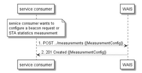
Figure 5.2.7.1-1: Flow of service consumer creating a measurement configuration
