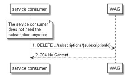
Figure 5.2.4.4-1: Flow of unsubscribing from the WLAN event notifications
