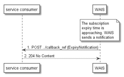
Figure 5.2.4.2-1: Flow of WAIS sending a notification on expiry of the subscription
