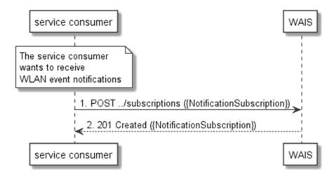
Figure 5.2.4.1-1: Flow of subscribing to WLAN event notifications
