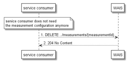
Figure 5.2.7.3-1: Flow of deletion of a Measurement Configuration
