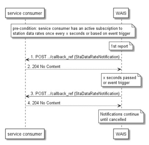
Figure 5.2.5-1: Flow of receiving WLAN event notifications on station data rates
