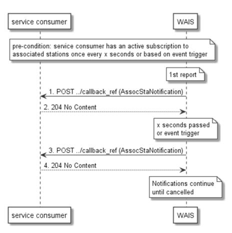
Figure 5.2.6-1: Flow of receiving WLAN event notifications on associated stations
