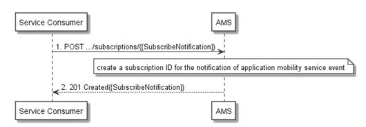
Figure 6.6-1: Flow of service consumer subscribing to notifications of Application Mobility Service events
