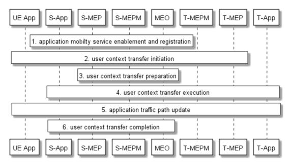
Figure 5.2-1: High level Application Mobility Service information flow
