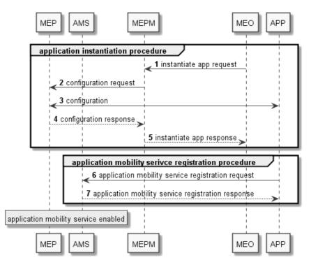
Figure 5.3-1: Application Mobility Service enablement and registration
