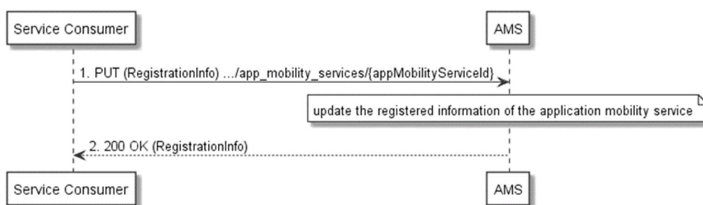
Figure 6.4-1: Flow of service consumer updating the registered Application Mobility Service
