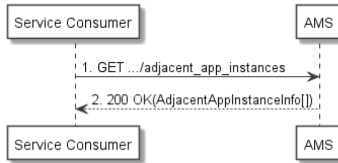
Figure 6.9-1: Flow of service consumer querying adjacent application instance information from AMS
