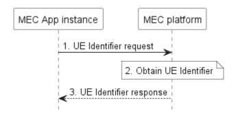
Figure 5.2.2.2-1: UE Identifier acquisition
