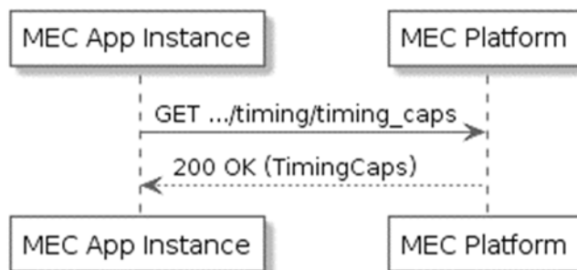
Figure 7.2.5.3.1-1: GET timing capabilities flow
