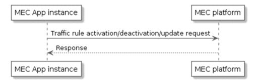
Figure 5.2.7-1: Flow of traffic rule activation/deactivation/update
