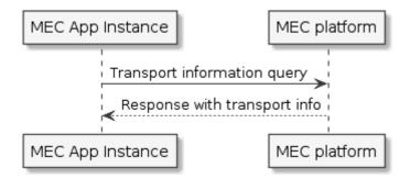
Figure 5.2.9-1: Flow of MEC application requesting transport information
