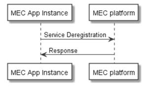
Figure 5.2.11-1: Flow of MEC service deregistration
