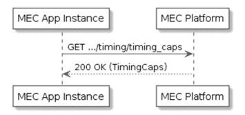
Figure 7.2.5.3.1-1: GET timing capabilities flow
