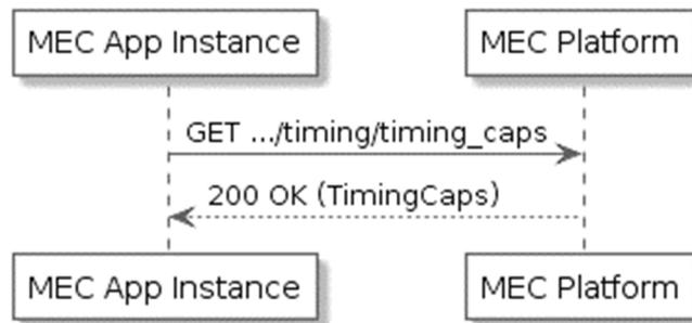
**Figure 7.2.5.3.1-1: GET timing capabilities flow**
