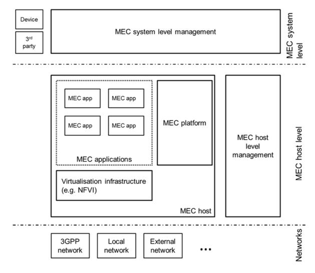
Figure 5-1: Multi-access Edge Computing framework
