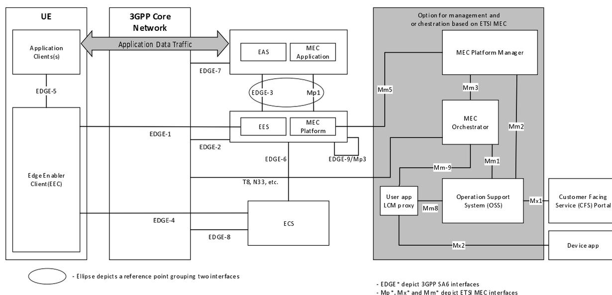
**Figure B.1-1: Relationship between 3GPP SA6 (EDGEAPP) architecture and ETSI MEC architecture, per the informative Annex C of ETSI TS 123 558 [i.9]**
