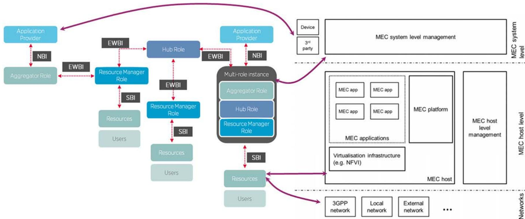
Figure C.1-1: Relationship between GSMA OP architecture and ETSI MEC framework, per Annex E.1.2 of [i.8]
