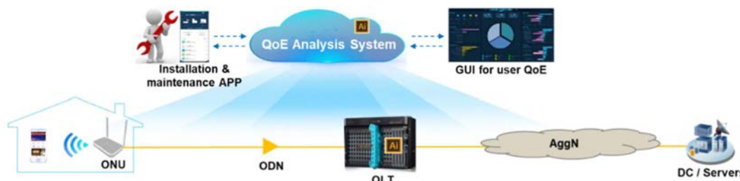
Figure 8: Overview of the F5G-A Residential broadband QoE evaluation and assurance (Source: ETSI GR F5G 020 [i.1])
