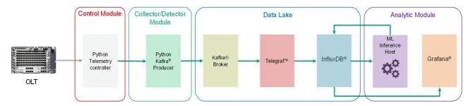
Figure B.1: Functional blocks of the proposed telemetry streaming workflow and ML pipeline
