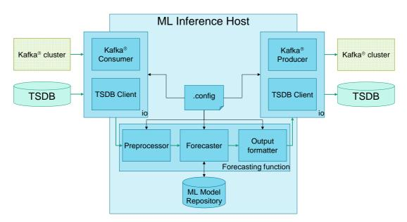
Figure B.7: Architecture of the ML inference host
