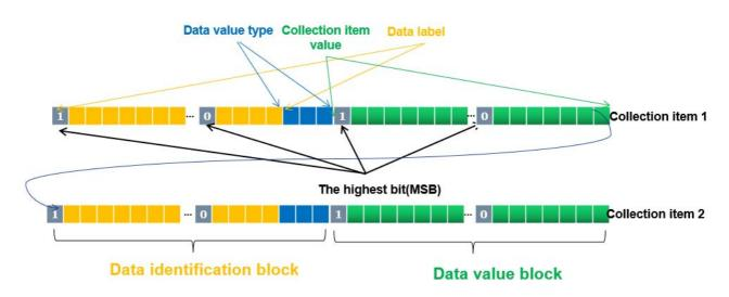
Figure C.1: Encoding Data Structure of Collection Items
