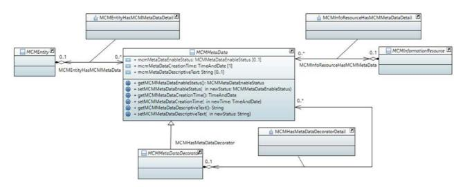
Figure 5-12: The MCMMetaData Hierarchy, Top Level View
