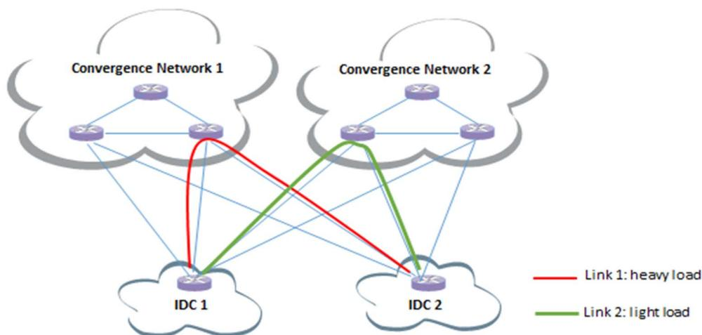
**Figure 5-1: Policy-driven, automatic IDC traffic steering**
