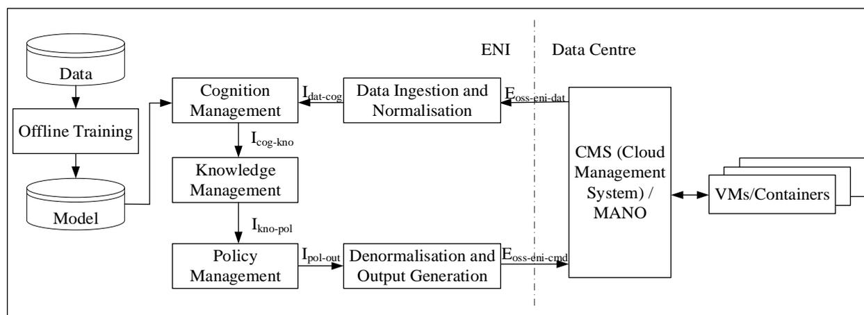
**Figure 5-3: Mapping to ENI reference architecture**
