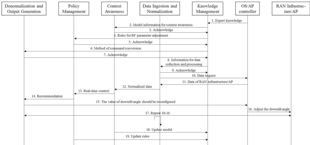
**Figure 5-8: Procedure for coverage and capacity optimization**
