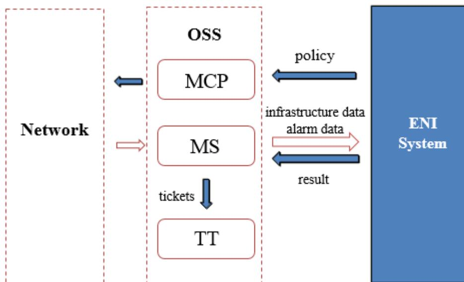
**Figure 5-29: Scenario of AI and ENI system enabled network fault root-cause analysis and intelligent recovery**
