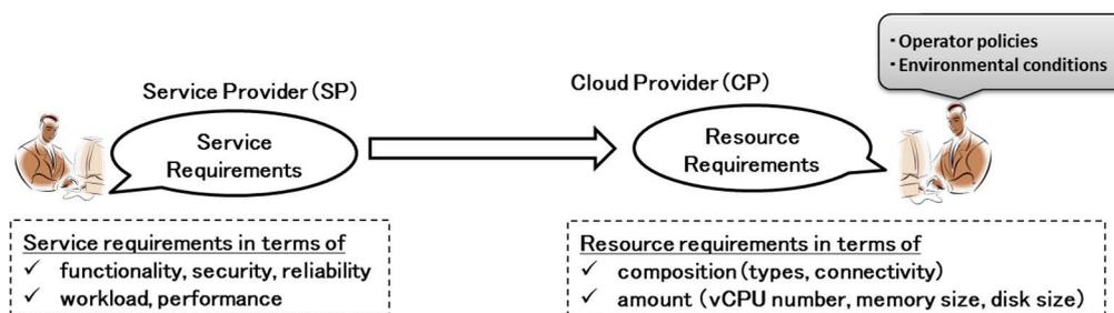
**Figure 5-17: Design cloud resources in accordance with service requirements**
