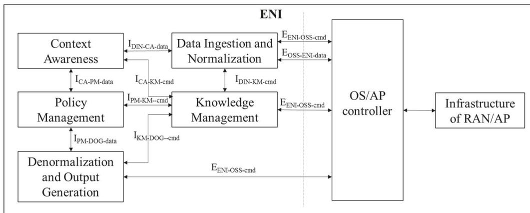
**Figure 5-7: Mapping to ENI reference architecture**
