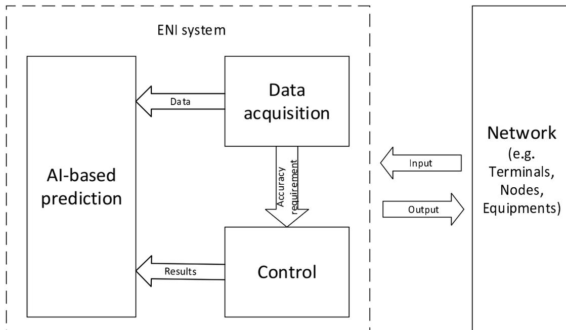
**Figure 5-19: Intelligent time synchronization of network**
