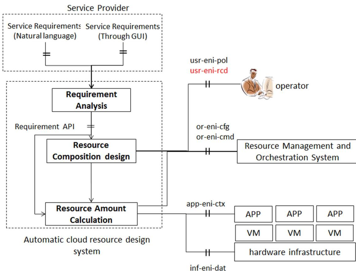
**Figure 5-18: Automatic Cloud Resource Design System**
