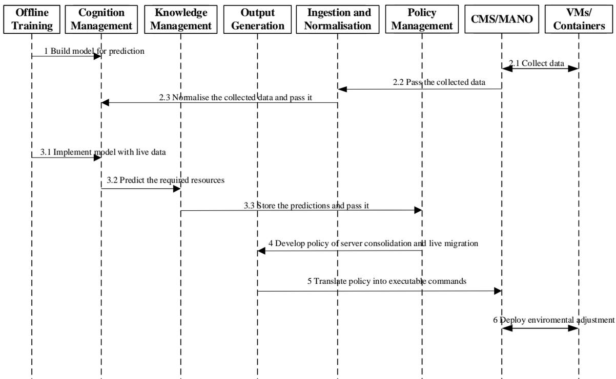
**Figure 5-4: Procedure for energy optimization using AI**
