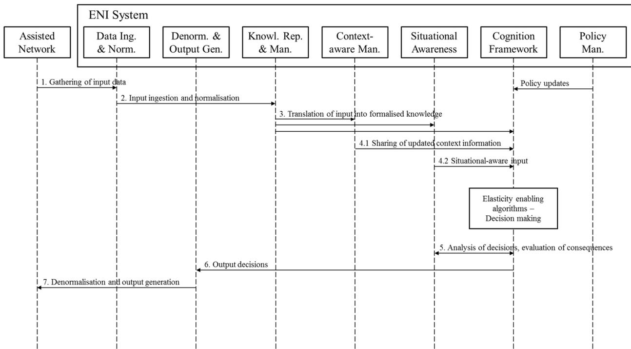
**Figure 5-10: Example Flow of information among the ENI System's functional blocks and the Assisted System**
