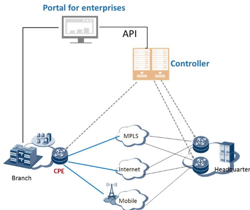
**Figure 5-24: Intelligent carrier managed SD-WAN service**
