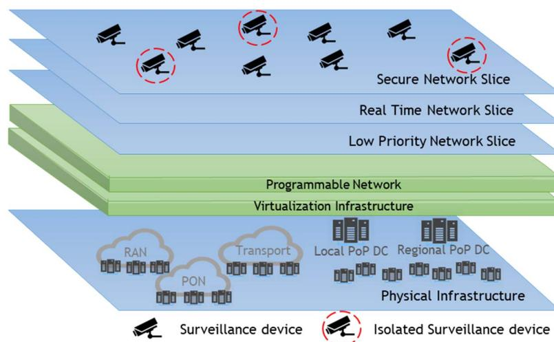
**Figure 5-30: Device isolation within a Network Slice**
