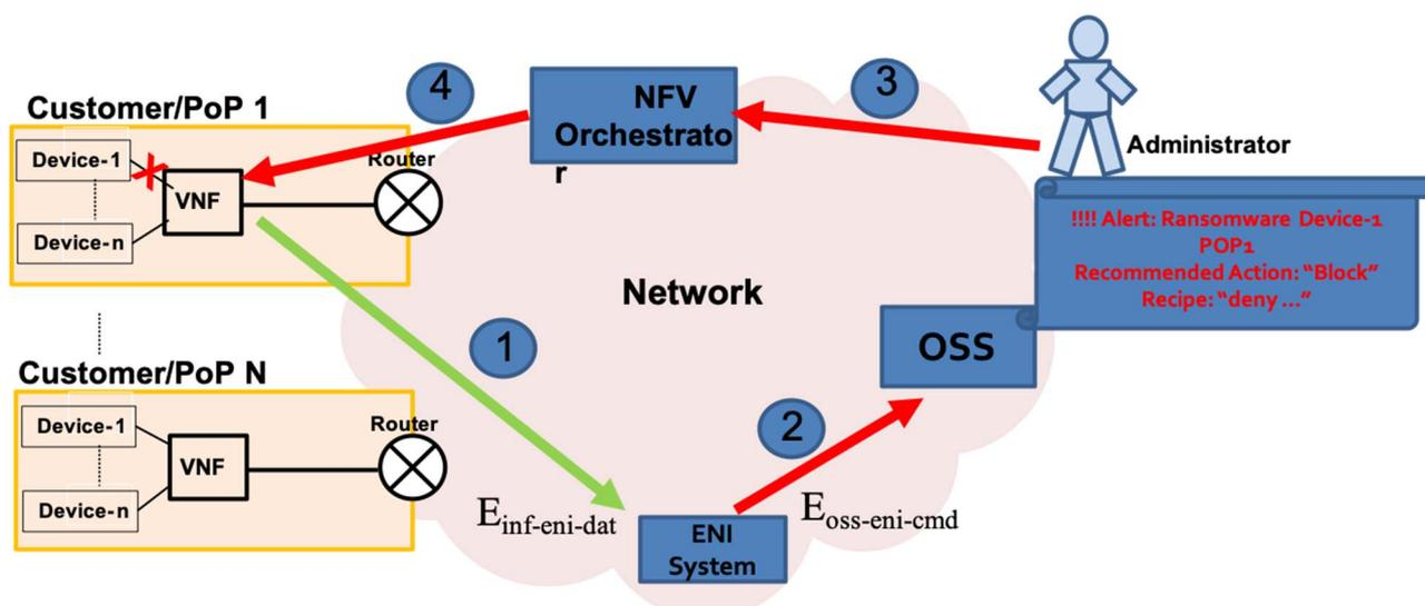
Figure 5-31: Use case to limit profit in cyber-attacks using NFV and ENI system
