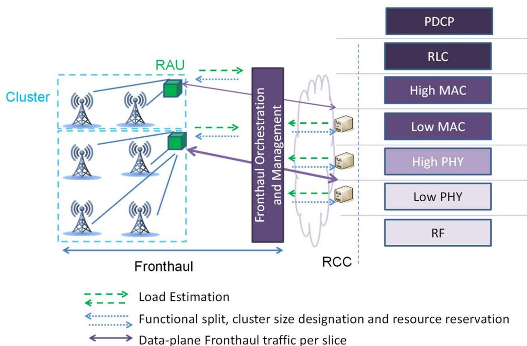
**Figure 5-9: Concept of the proposed Fronthaul use case**
