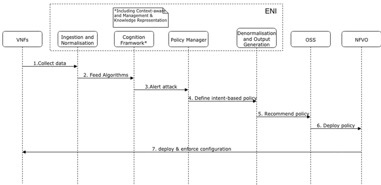
**Figure 5-32: Flow of information among the ENI System's functional blocks and the Assisted System**
