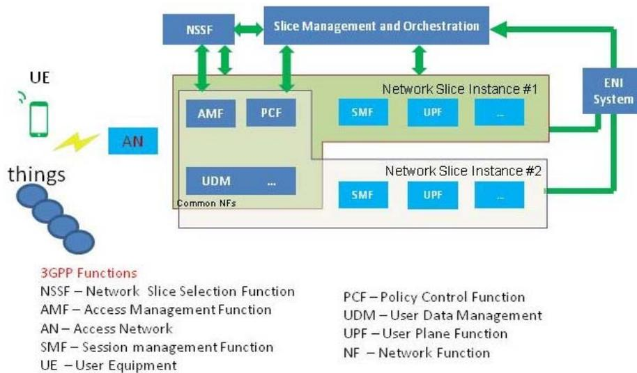
**Figure 5-23: Example of a network slicing management and orchestration scenario**
