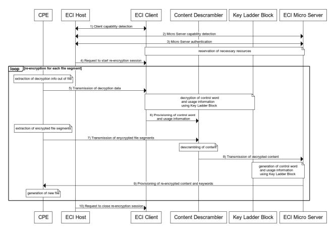
Figure 9-1: Flow diagram for the re-encryption of content
