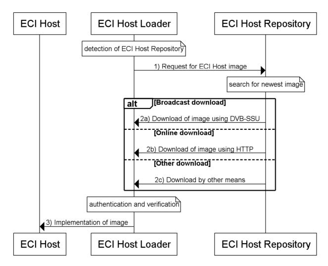
Figure 5-1: Flow diagram for the installation of an ECI Host
