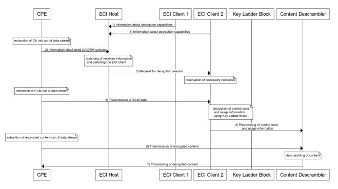
Figure 8-1: Flow diagram for the decryption of content
