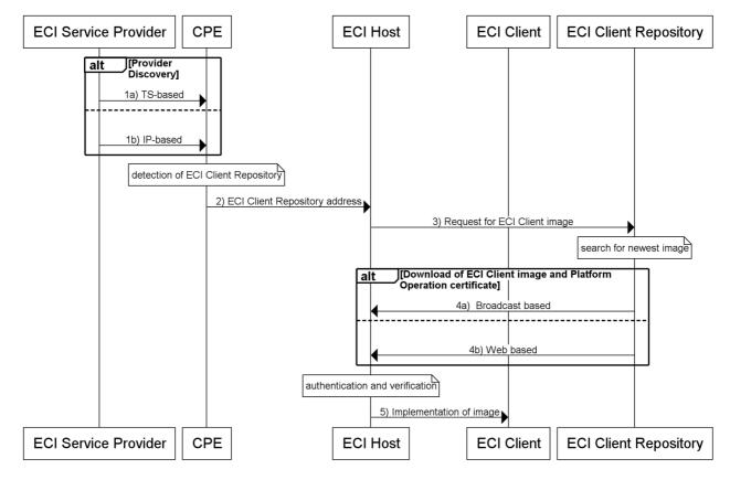
Figure 6-1: Flow diagram for the installation of an ECI Client
