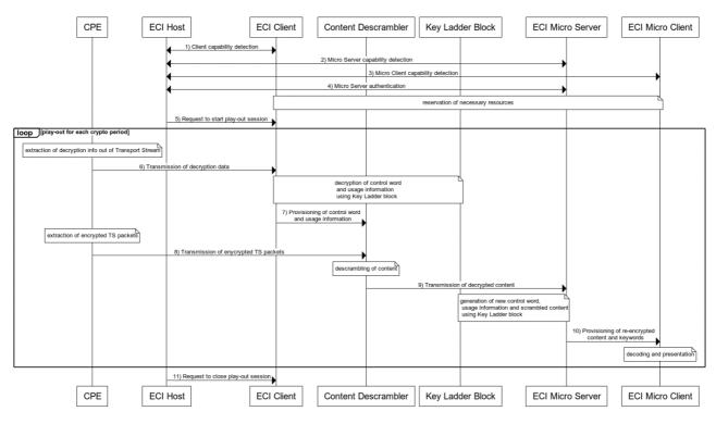
Figure 10-1: Flow diagram for the play-out of content
