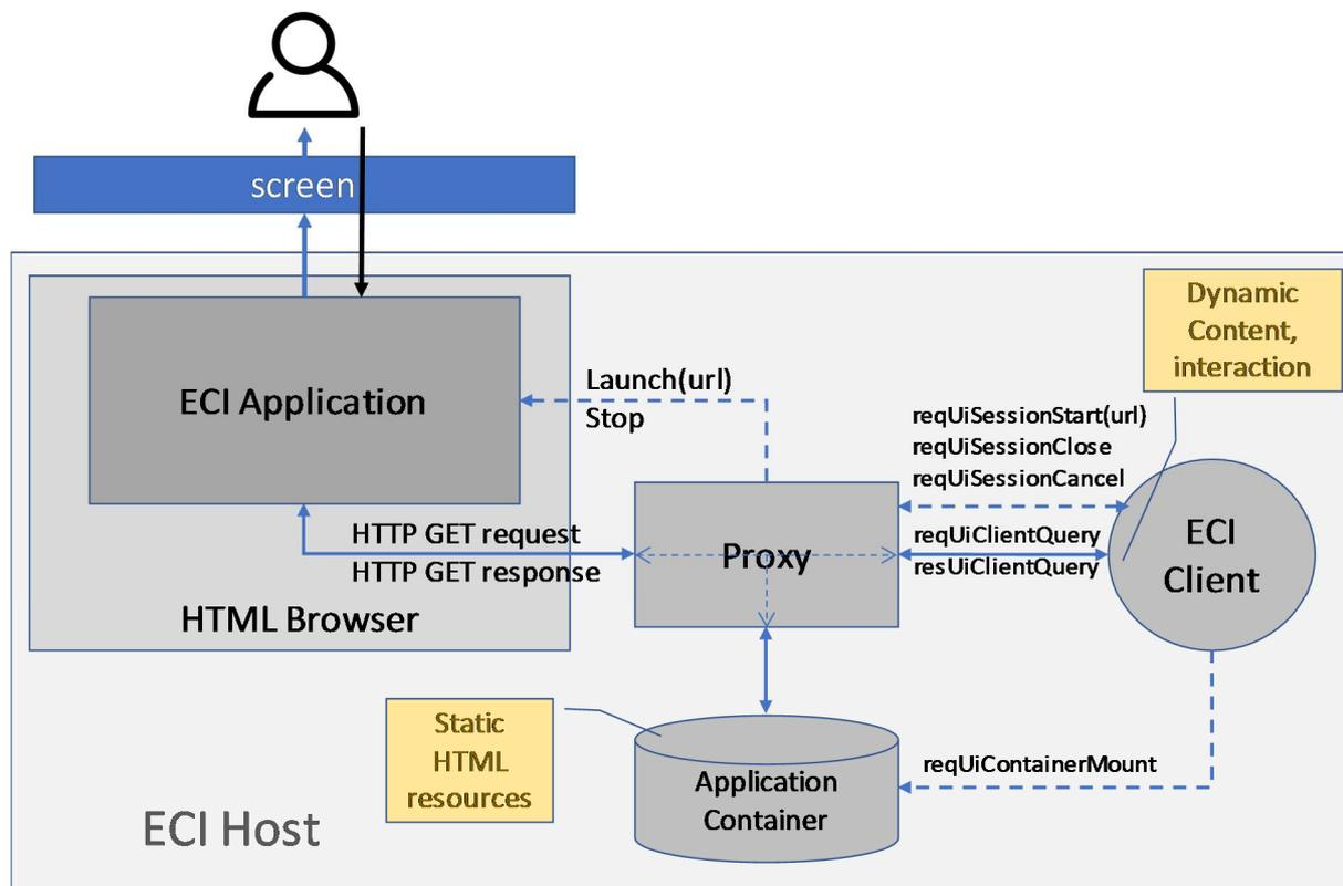
Figure 9.4.3.1-1: Block diagram of the User Interface API
