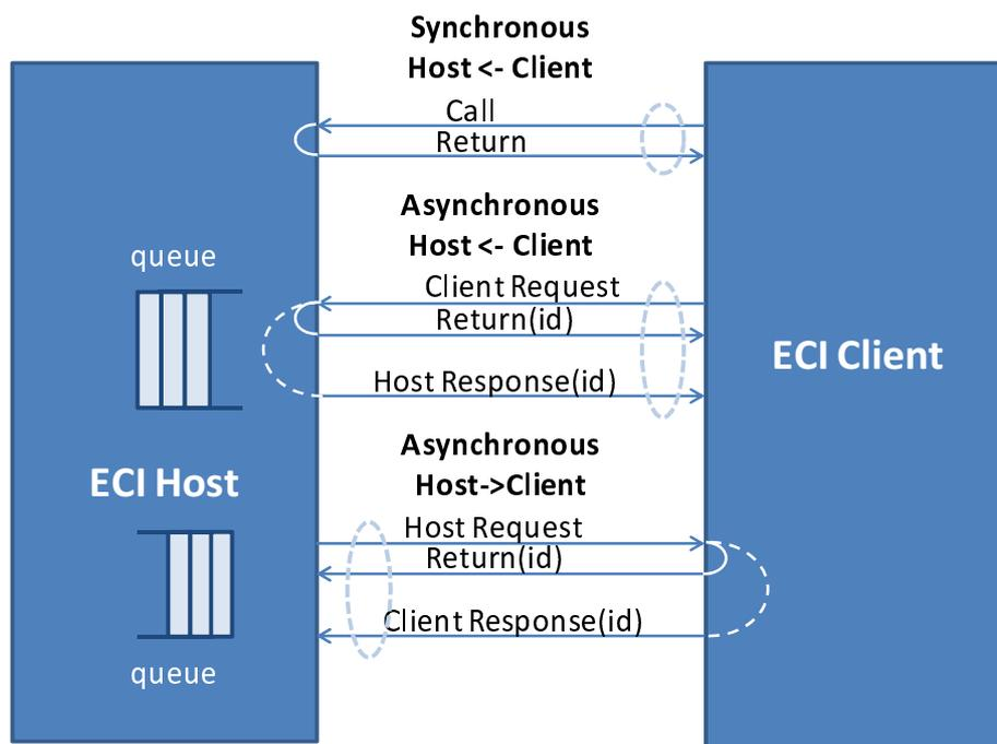
**Figure 9.2.3-1: Message exchanges between Client and Host**
