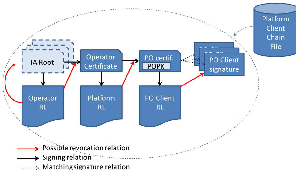
Figure 7.5.1-1: Authentication chain for the platform client chain
