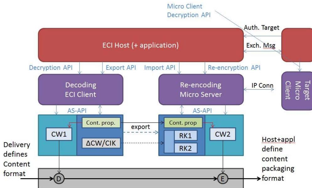
**Figure 9.7.1.3-1: Architecture of the decryption and re-encryption functionalities**
