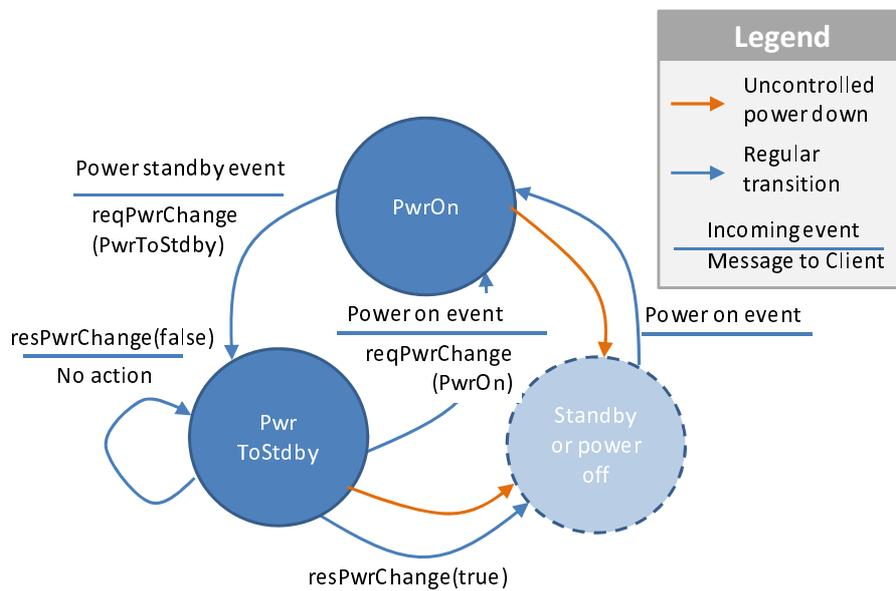
Figure 9.4.7.1-1: ECI Host power states and main interaction with a managed Client
