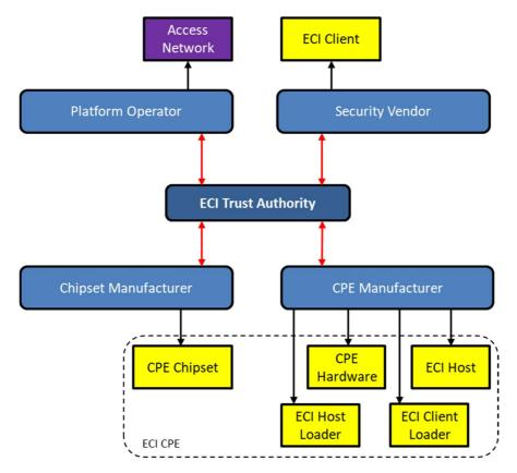
Figure 4: Necessary trust management between Trust Authority and the relevant stakeholders in a Trust Environment
