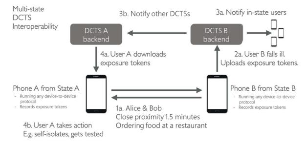
Figure 3: End-to-end DCTS exposure notification flow
