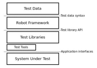
Figure 1: Robot Framework architecture
