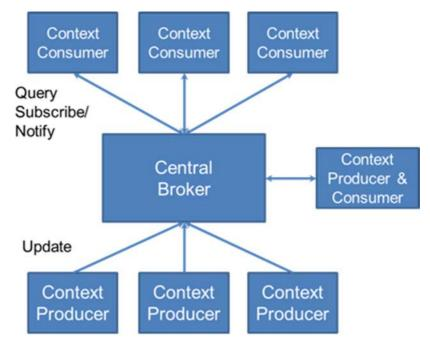
Figure 4.3.2-1: Centralized architecture
