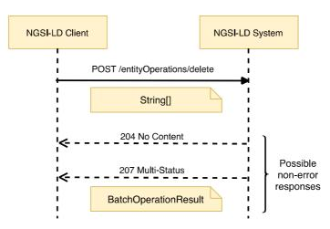
Figure 6.17.3.1-1: Batch Entity Delete Interaction
