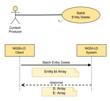
Figure 5.6.10.2-1: Delete a batch of Entities use case
