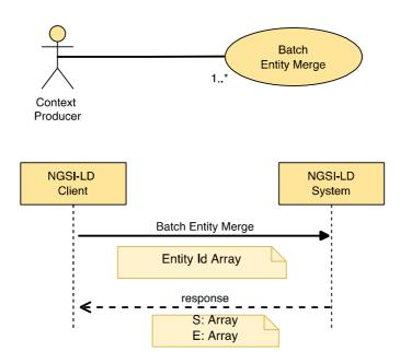
Figure 5.6.20.2-1: Merge a batch of Entities use case
