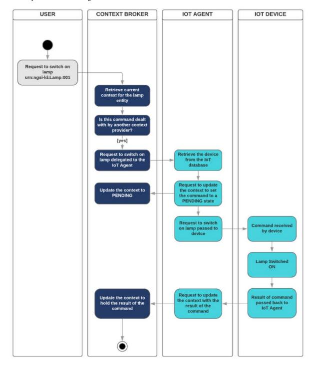
Figure H.6-1: IoT Agent node library implementation of the NGSI-LD system and actuation workflow
