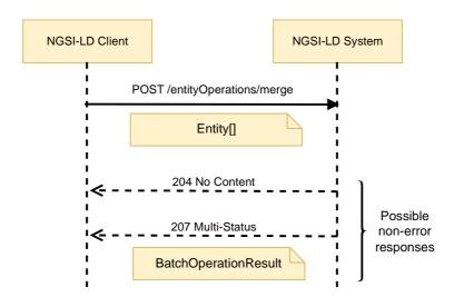
Figure 6.31.3.1-1: Batch Entity Merge Interaction
