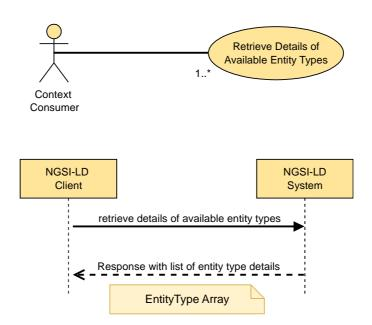
Figure 5.7.6.2-1: Retrieve Details of Available Entity Types use case
