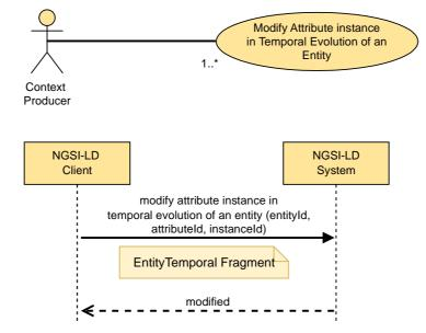
Figure 5.6.14.2-1: Modify Attribute Instance in Temporal Evolution of an Entity use case
