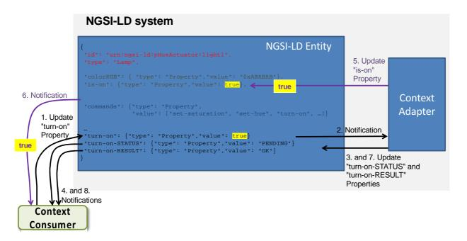
Figure H.4.2-1: Steps of the actuation workflow using subscription/notification
