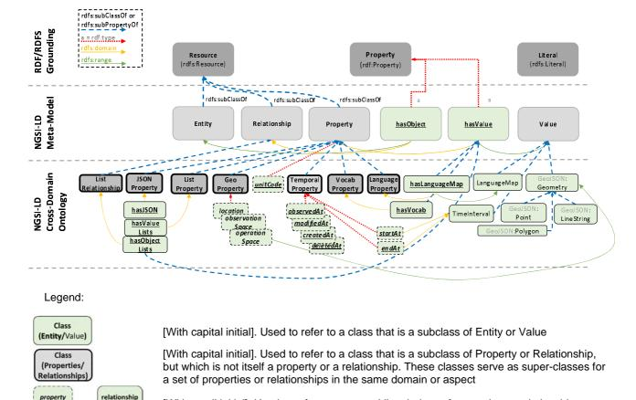
Figure 4.2.3-1: NGSI-LD Core Meta-Model plus the Cross-Domain Ontology
