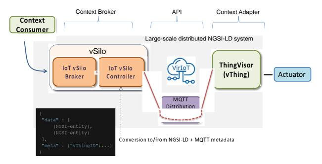
Figure H.5-1: VirloT implementation of the NGSI-LD system and actuation workflow
