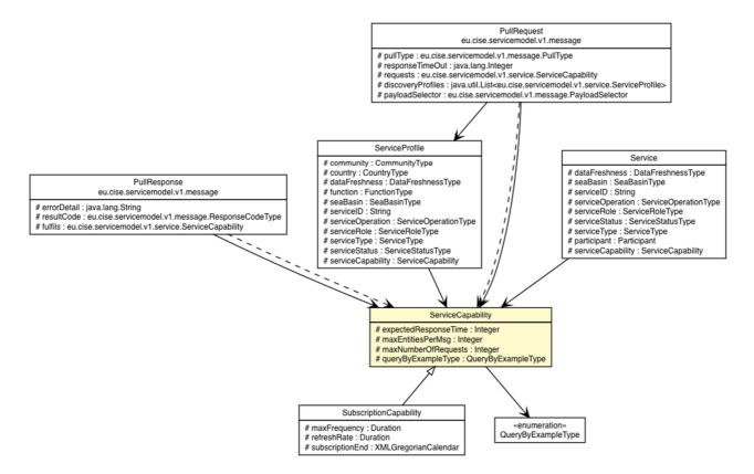
Figure 15: ServiceCapability class diagram
