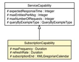
Figure 17: SubscriptionCapability class diagram
