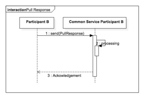
Figure 39: Common Services pull response operation
