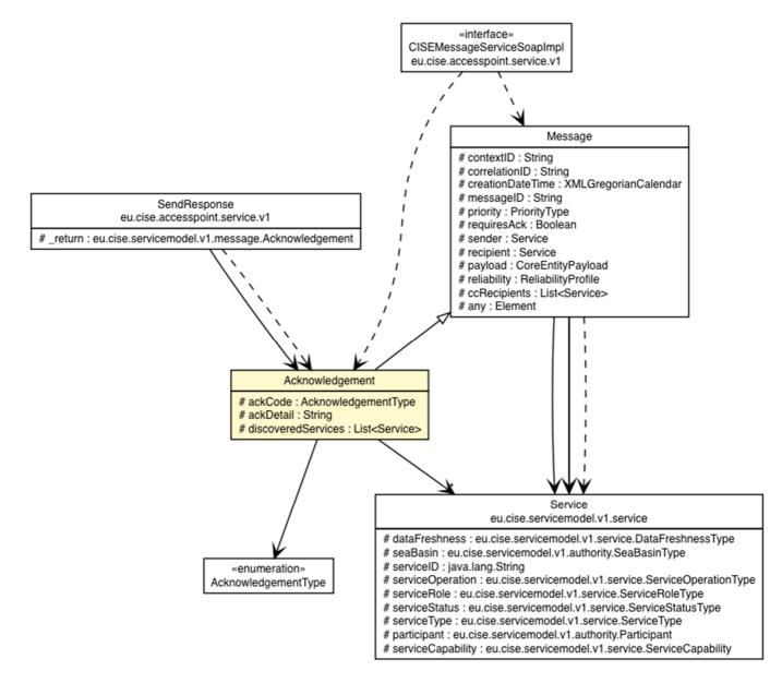
Figure 23: Acknowledgement class diagram
