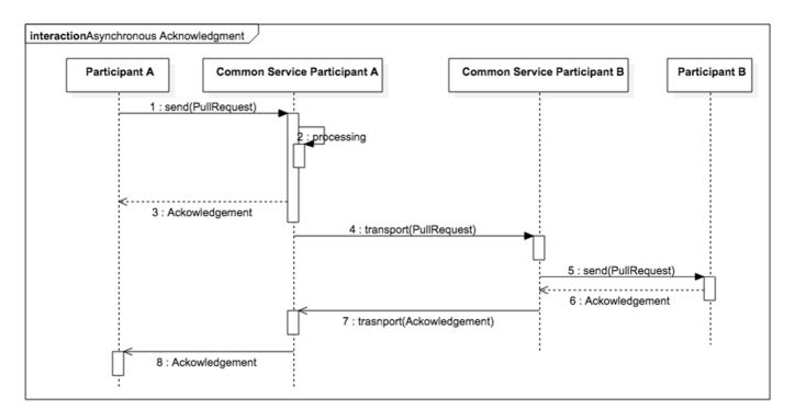
Figure 50: Common Services asynchronous acknowledgment
