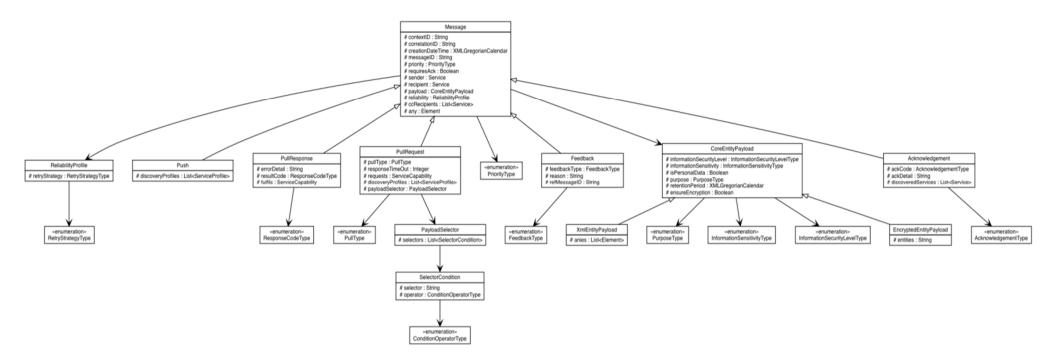
Figure 19: MESSAGE package class diagram
