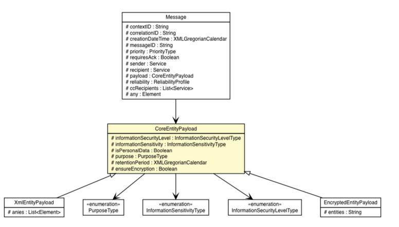
Figure 29: CoreEntityPayload class diagram
