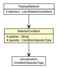
Figure 33: SelectorCondition class diagram
