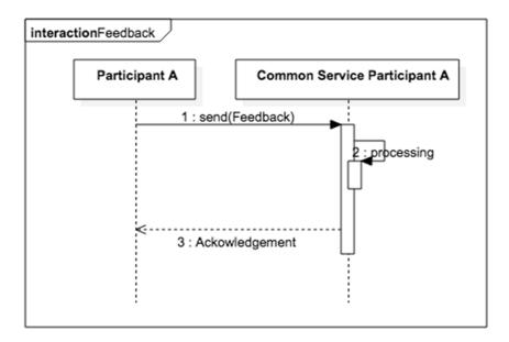
Figure 42: Common Services feedback operation
