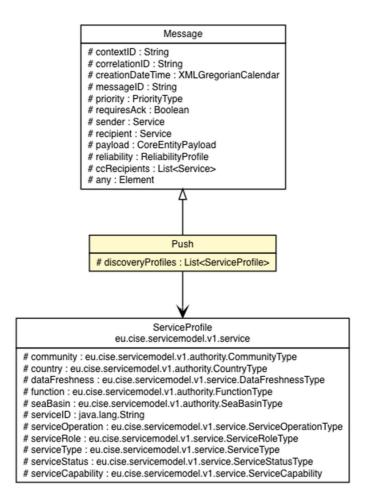
Figure 22: Push class diagram
