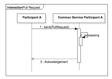
Figure 38: Common Services pull request operation
