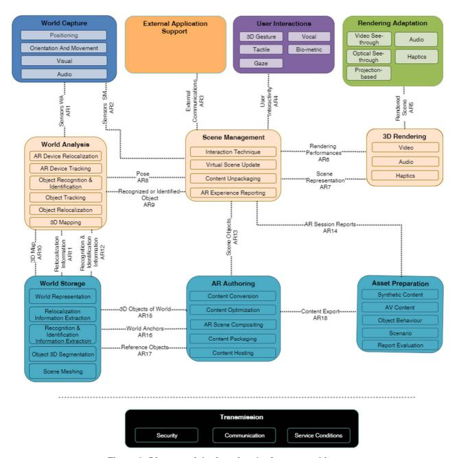
Figure 2: Diagram of the functional reference architecture
