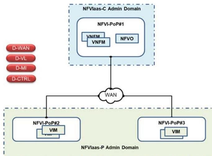
**Figure 5.4.4-1: NFV-MANO deployment in multi-site environment with the NFVIaaS-C's NFV-MANO functions located in the same NFVI-PoP**
