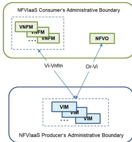
**Figure 5.4.2-2: NFVlaaS-C Management Functions interacting with NFVlaaS-P's VIM(s) via MLPOC in direct mode**
