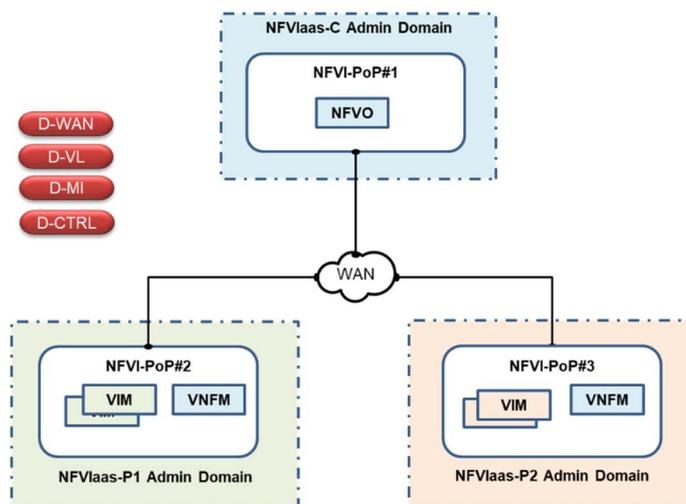
**Figure 5.4.4-3: NFV-MANO deployment in multi-site environment with the NFVlaaS-C managing NS deployed across different NFVlaaS-P's administrative domains**
