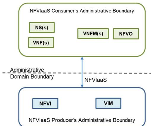
**Figure 5.4.2-1: Relationship between NFVIaaS-P and NFVIaaS-C (ETSI GR NFV-IFA 028 [i.2])**
