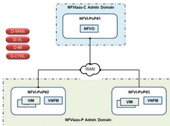
**Figure 5.4.4-2: NFV-MANO deployment in multi-site environment with the NFVIaaS-C's NFV-MANO functions distributed in different NFVI-PoPs**
