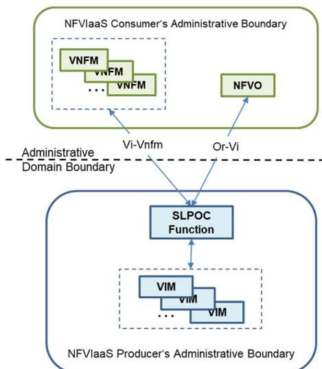
**Figure 5.4.2-4: NFVlaaS-C Management Functions interacting with NFVlaaS-P's VIM(s) via SLPOC in direct mode**
