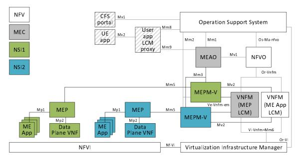
Figure 5.5.1-1: Example of MEC in NFV with dedicated instances of MEC components in distinct NSIs
