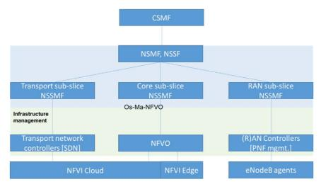
Figure 5.3.1-1: Network Slice architecture including MEC
