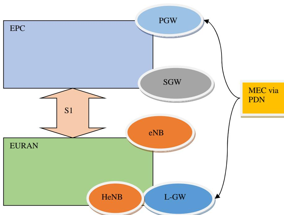
Figure 6.2.7.1-1: Potential attach points of MEH in LTE/EPC network
