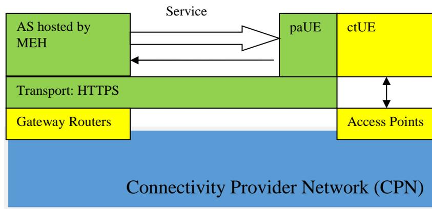
**Figure 6.1.1-1: Illustration of relations of components in MEC for service provisioning**
