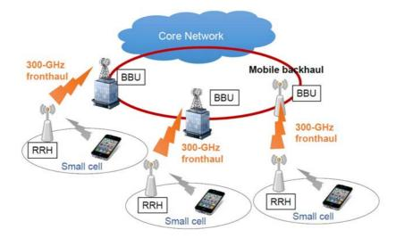
Figure 14: Example of fronthauling and backhauling in mobile network architecture (Source: Report ITU-R SM. 2450-0 [i.12])
