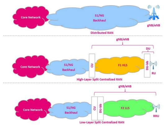
Figure 12: Distributed and Centralized RAN Architectures
