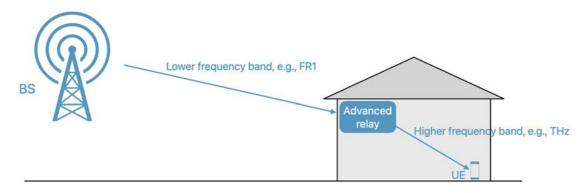
Figure 37: Advanced relay assisted transmission for indoor user
