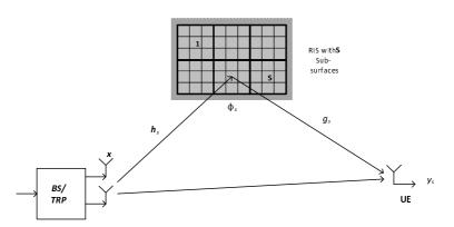
Figure 23: System model for sub-surface based RIS channel estimation
