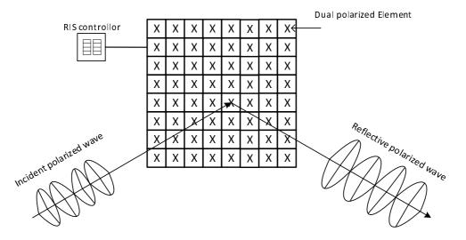
Figure 17: Dual polarized RIS
