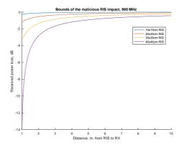
Figure 13: Destructive beamforming upper bounds, 0,9 GHz band
