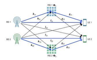
Figure 11: Example scenario - Two links aided by two RIS
