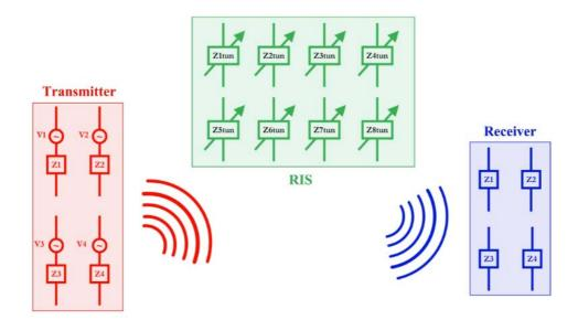
Figure 1: Mutually coupled antenna model
