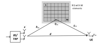
Figure 22: System model for element wise RIS channel estimation
