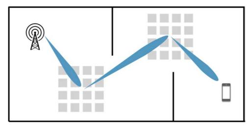
Figure 29: Cascading RIS links assist UEs to form links with BSs regardless of blockage
