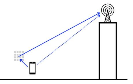
Figure 37: Scenario II - UE-controlled RIS to provide diversity gain against UE's rotation and self-blockage
