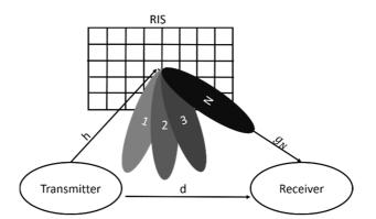
Figure 24: System model for configuration-wise RIS channel estimation
