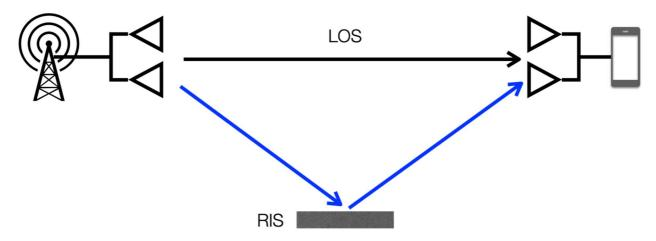
Figure 32: Utilizing RIS with MIMO: multiplexing and interference management
