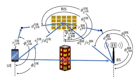
Figure 5: RIS localization scenario with MIMO system
