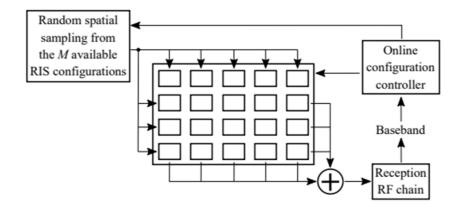
Figure 25: Block diagram of the proposed RIS hardware architecture including a single active reception RF chain for explicit channel estimation at the RIS side
