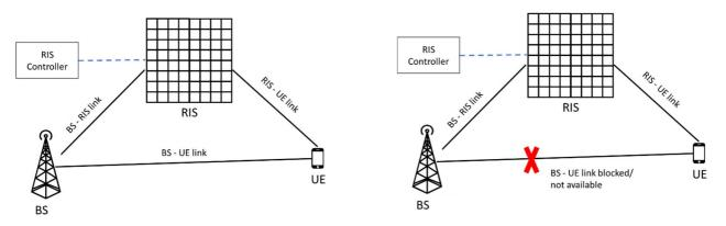
Figure 20: Scenarios for RIS-aided channel estimation based on the availability of the direct link between BS-UE
