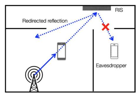
Figure 33: Utilizing RIS for secure communication
