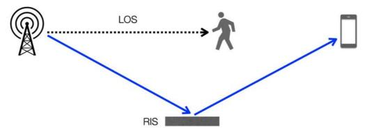
Figure 27: RIS as a solution to blockage
