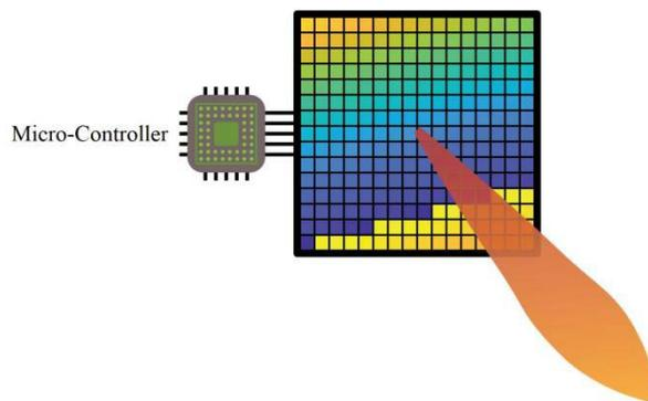
**Figure 5.1-1: Illustration of a RIS comprising a micro-controller and a panel**
