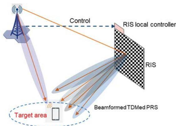
**Figure 6.2.3.2-2: Topology of the RIS-integrated localization with single BS/single RIS**
