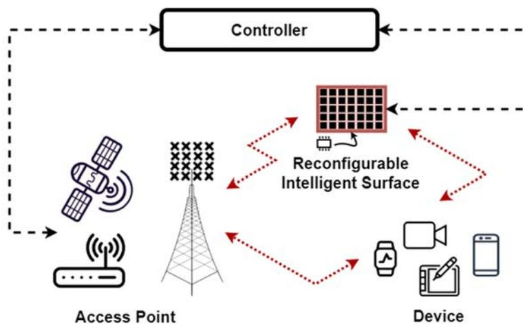
**Figure 4.1-1: Illustration of deployment scenario of RIS**
