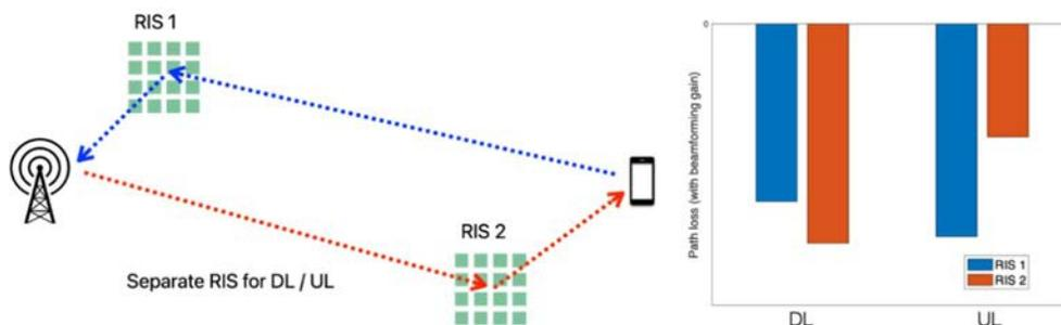
**Figure 6.3.2.2-2: Using separate DL/UL RIS.**
