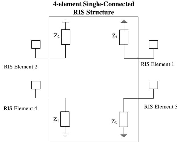
**Figure 5.2.1.1.1-1: Single-connected impedance-based RIS structure**
