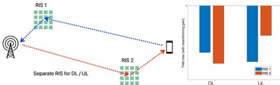
**Figure 6.3.2.2-2: Using separate DL/UL RIS.**
