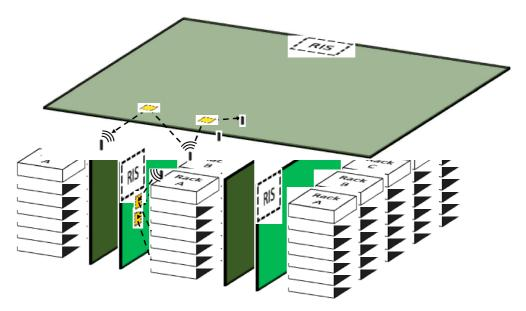
Figure 5.8.1-1: Programmable wireless data centers with RIS installed
