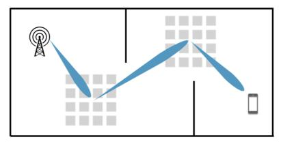
Figure 5.1-3: Cascading RIS links assist UEs to form links with BSs regardless of blockage
