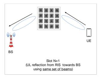
Figure 4.5.1-1(a): Illustration of TDD communication with reciprocity-constrained mode at UE using same set of phase shifts for UL and DL at RIS
