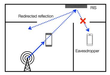
Figure 5.4-1: Utilizing RIS for secure communication
