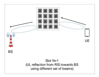
Figure 4.5.1-1(b): Illustration of TDD communication with reciprocity-non-constrained mode at UE using different set of phase shifts for UL and DL at RIS
