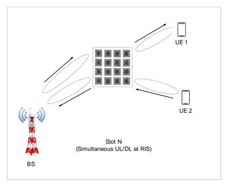
Figure 4.5.3-1: Illustration of full-duplex mode at RIS
