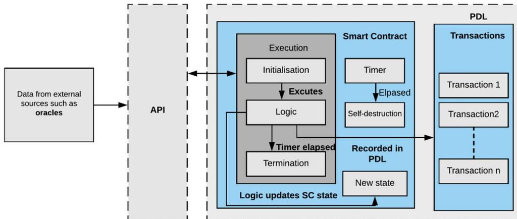
Figure 6-2: Reference Architecture of a Smart Contract without contract chaining
