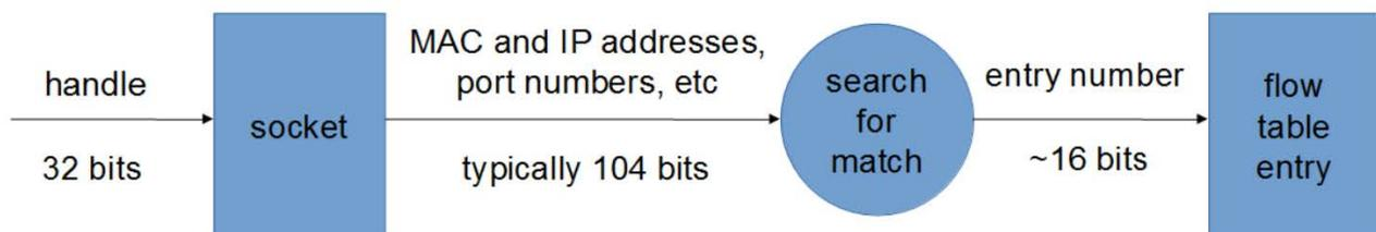
**Figure 9.2: Flow identification in current networks**
