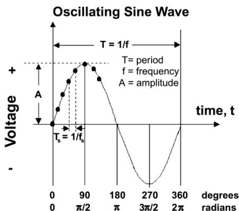
**Figure 4.1: Characteristics of a sinusoidal wave**
