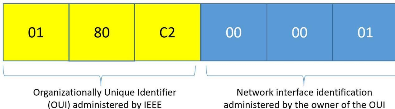
**Figure 5.5: Structure of a MAC address**
