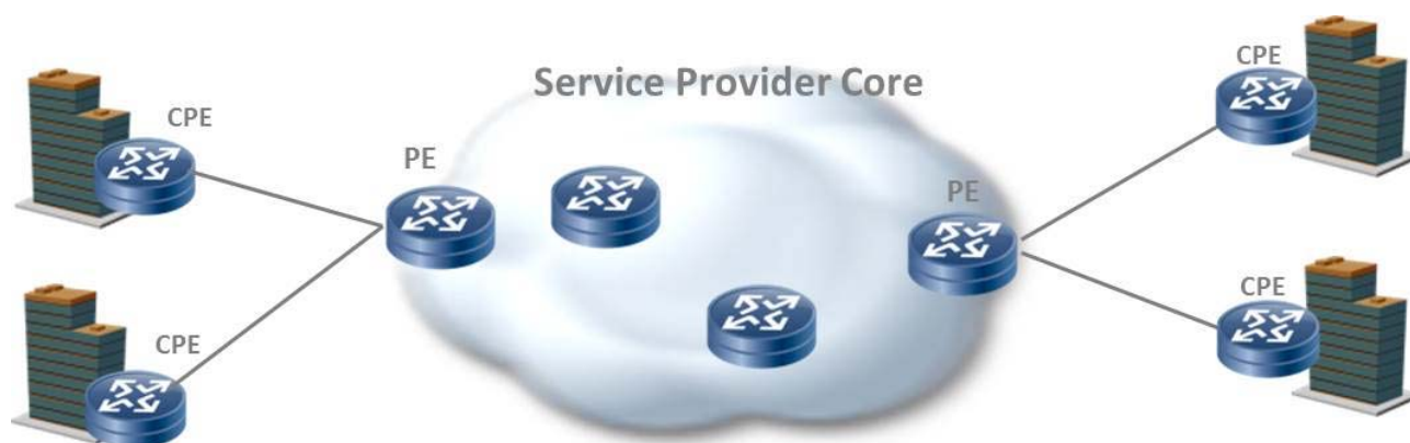
Figure 6.2.2-1: Service Provider without virtualisation of the enterprise
