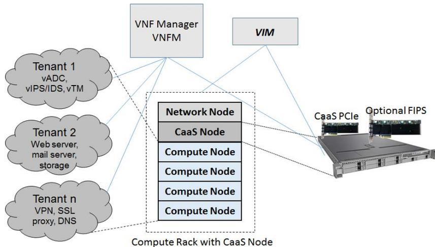
**Figure 19: Crypto as a Service (CaaS) deployed as a shared network resource (e.g. part of NFVI)**
