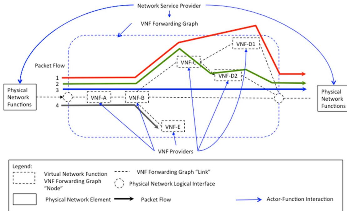
**Figure 5: Logical View of Virtual Network Function Forwarding Graph (VNF FG)**
