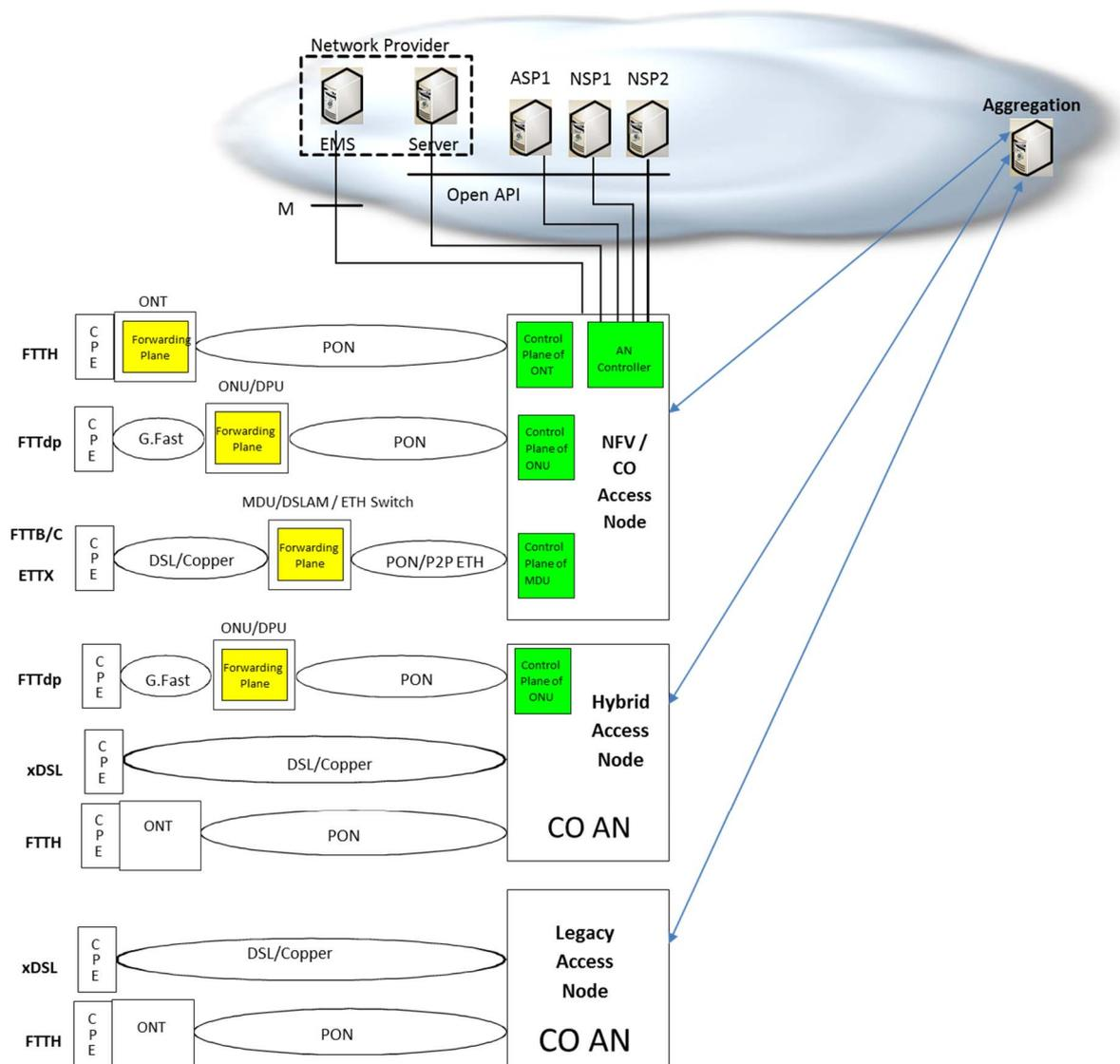
Figure 18: Virtualised and Legacy Access Networks (DSL and FTTP example)
