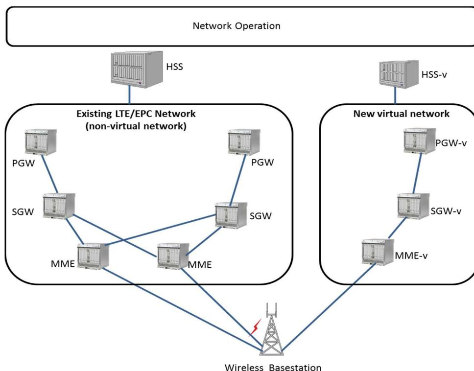
**Figure 7: An example of coexistence of virtual and non-Virtualised mobile core networks**
