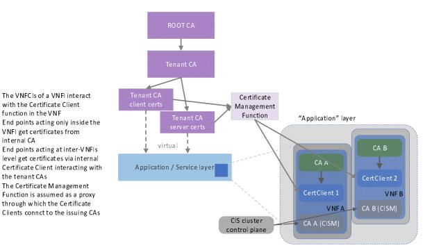
Figure 10.5.4-1: Certificate Client and Certificate Management Function in cooperation to provide certificates
