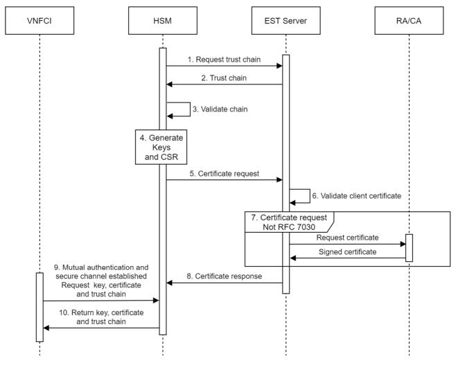
Figure 8.1.2.3-1: HSM certificate enrolment for VNFCI procedure
