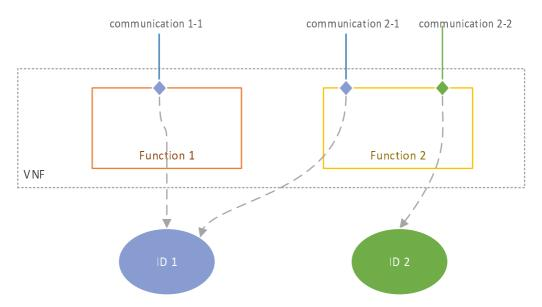
Figure 9.2.1.1-1: Mapping between function and ID
