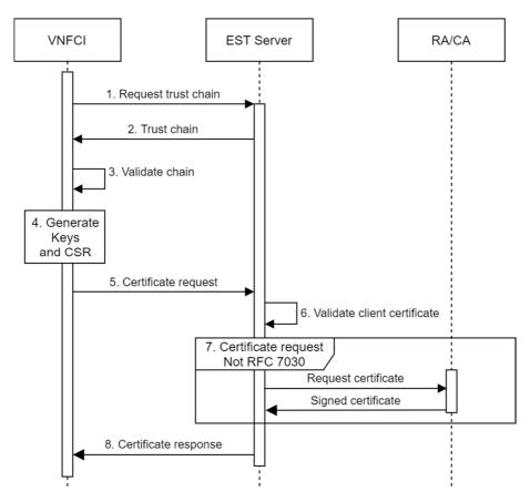
Figure 8.1.2.1-1: Direct VNFCI certificate enrolment procedure
