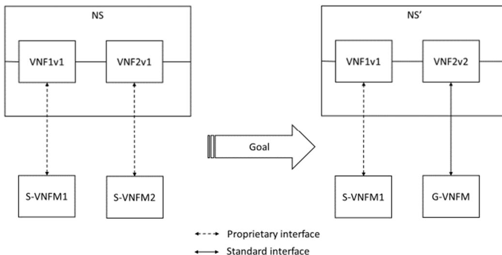
**Figure 5.5.2.1-1: Use case of replacing a S-VNFM with a G-VNFM with standard interface**
