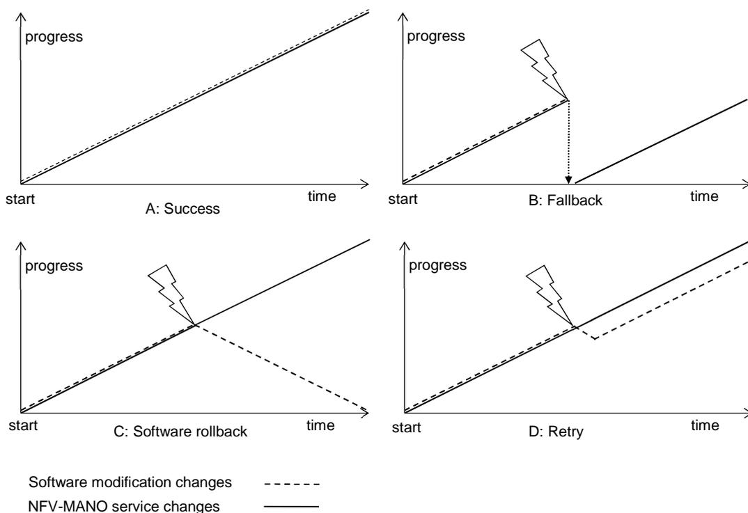
**Figure 4.1.3-1: Fallback, rollback and retry of the software modification process**
