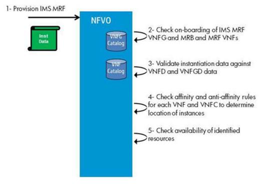
Figure A.5: IMS MRF deployment - initial steps
