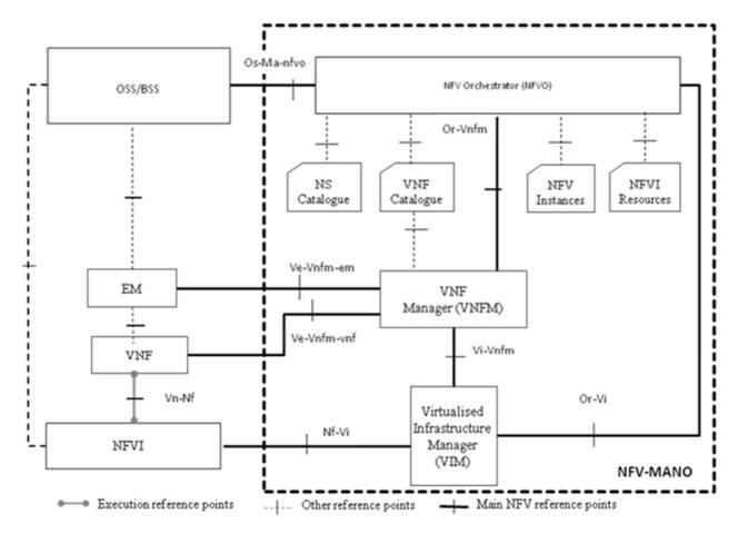
Figure 5.1: The NFV-MANO architectural framework with reference points
