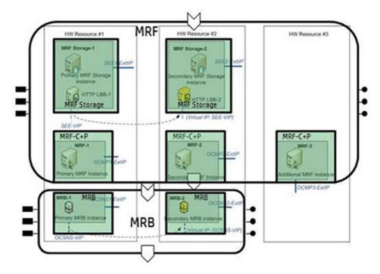
Figure A.2: IMS MRF target deployment
