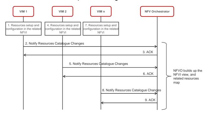
Figure D.1: NFVI-PoP setup and configuration flow
