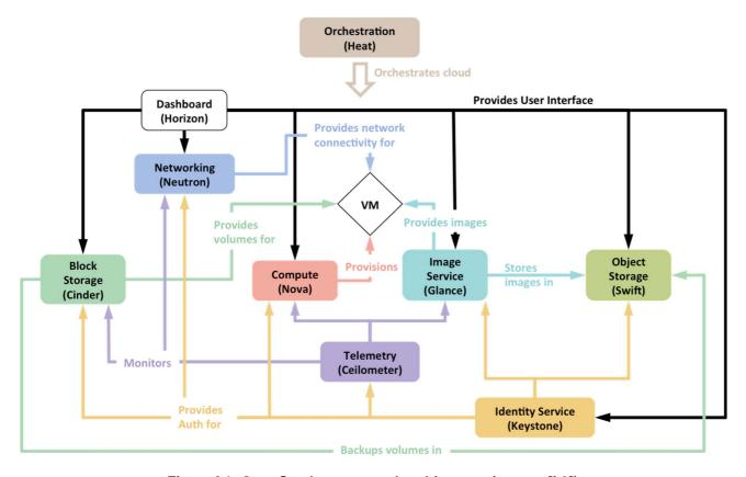
Figure I.1: OpenStack conceptual architecture (source [i.9])
