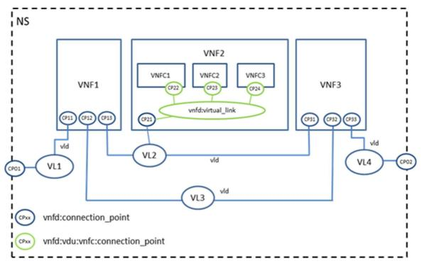
Figure 6.4: Relationships between internal and external Virtual Links
