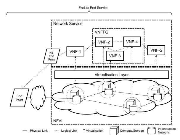
Figure 6.6: Example of a Network Service as part of an end-to-end service with VNFs and a forwarding graph
