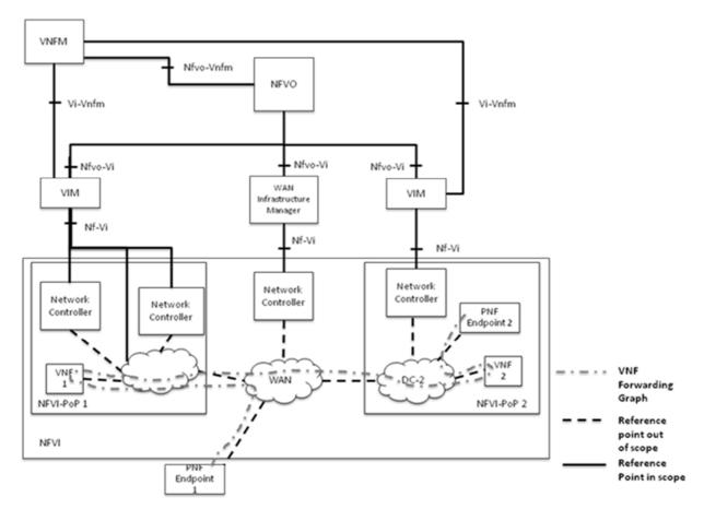
Figure 5.2: Network Controller example
