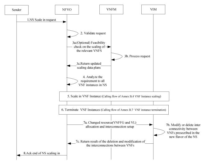
Figure C.10: Network Service scaling in message flow
