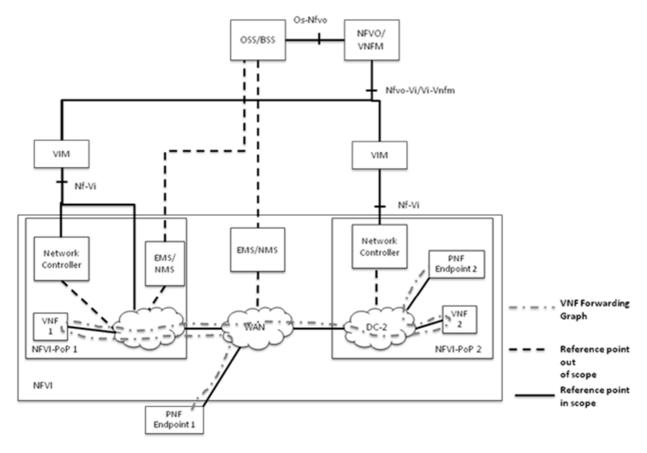
Figure 5.3: EMS/NMS for the NFVI network
