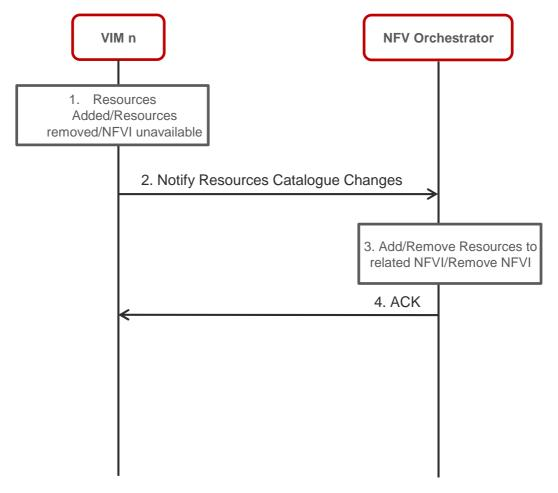
Figure D.2: Resources provisioning/de-provisioning flow
