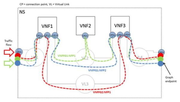
Figure 6.5: Network Service with two VNFFGs with different NFPs
