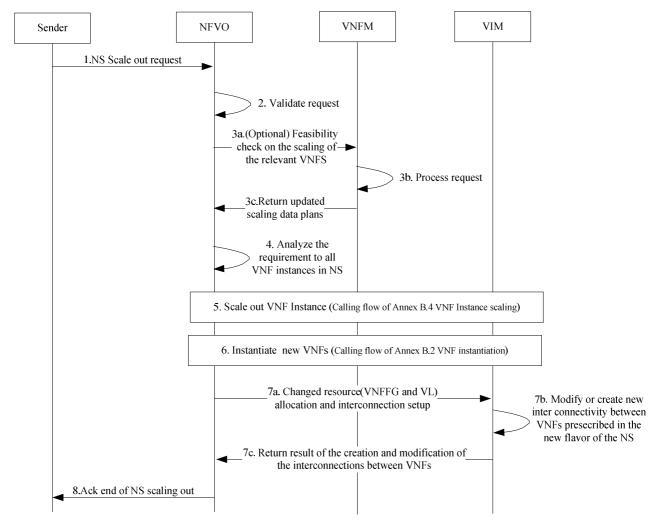
Figure C.9: Network Service scaling out message flow
