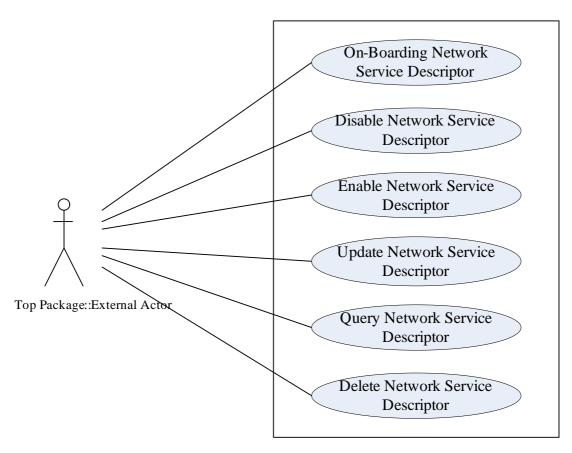
Figure C.1: Use case diagram for Network Service on-boarding
