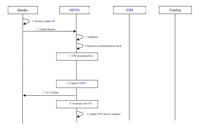
Figure C.12: NS instance update due to VNF instance modification flow
