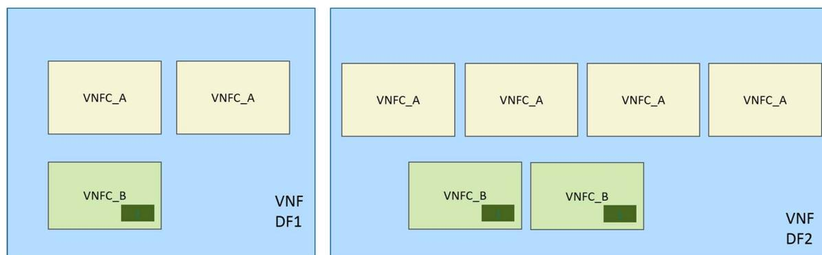
**Figure A.2-1: Example of a VNF with licensing based on number of VNFC instances with different deployment flavours**
