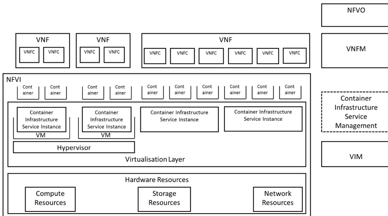
**Figure 5.3.6.1-1: NFVI provides containers on bare metal and VM**
