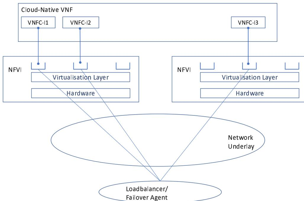
**Figure 5.2.2.1-1: An example to illustrate n+k redundancy with load-balancing between distributed VNFC instances**
