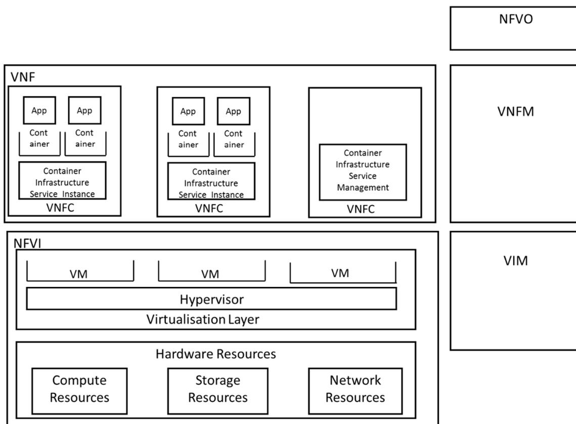
Figure 5.3.2.1-1: Containerized NFV Micro-Services within the VNF
