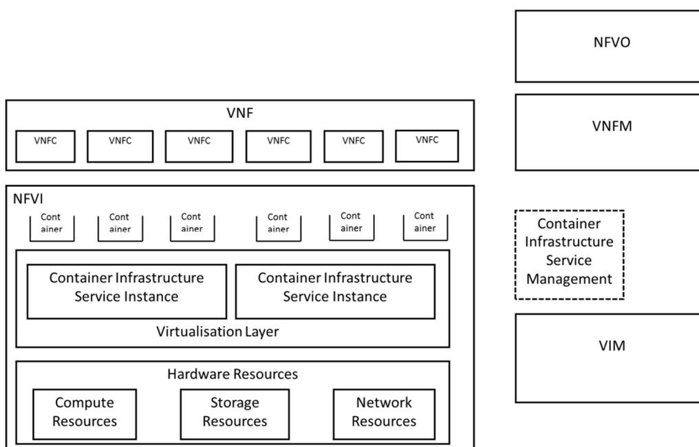
**Figure 5.3.3.1-1: Illustration of VNFC in container on bare metal**
