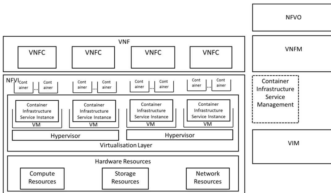
**Figure 5.3.5.1-1: Illustration of VNFC in group of containers**
