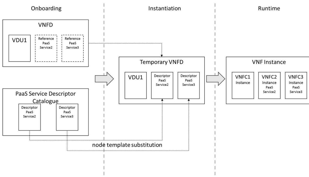
**Figure 5.1.8.1-2: Stages for instantiating a VNF using PaaS service descriptors**
