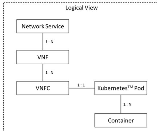
Figure 6.2.4-1: Example logical model mapping for Kubernetes®
