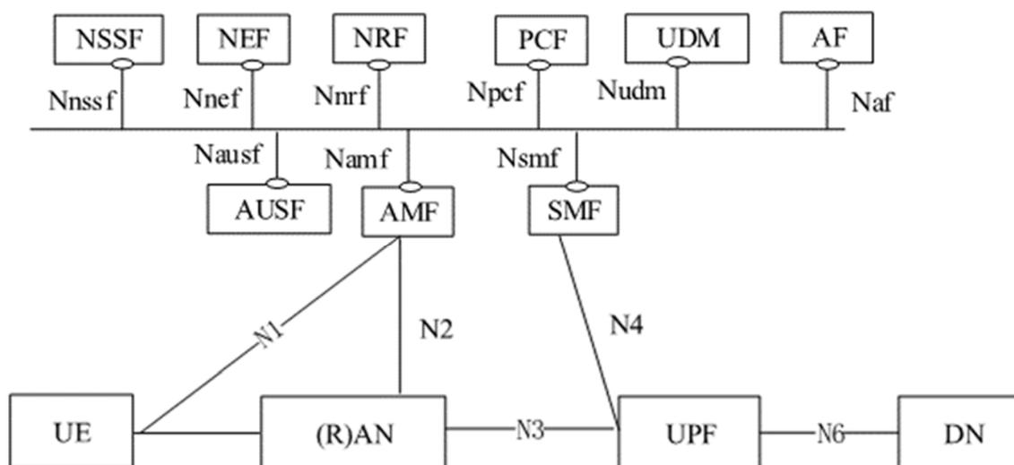
**Figure 5.1.7.1-1: (Non-roaming) 5G System Service-based architecture**
