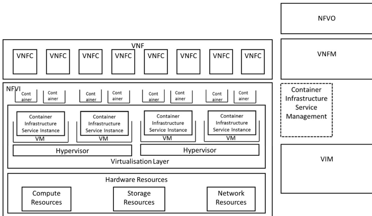
**Figure 5.3.4.1-1: Illustration of VNFC in container in virtual machine**
