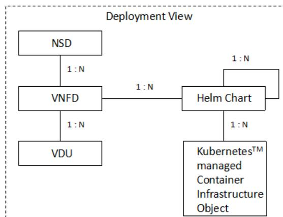
Figure 6.2.4-2: Example deployment object mapping for Kubernetes® and Helm™
