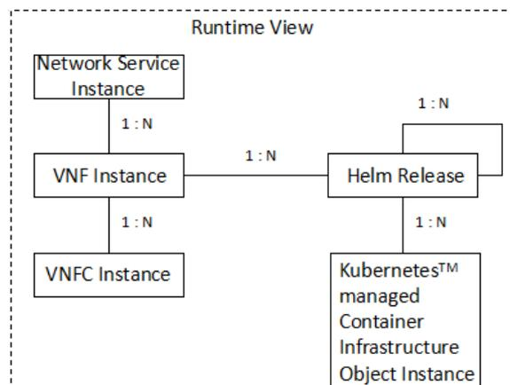
Figure 6.2.4-3: Example runtime object mapping for Kubernetes® and Helm™
