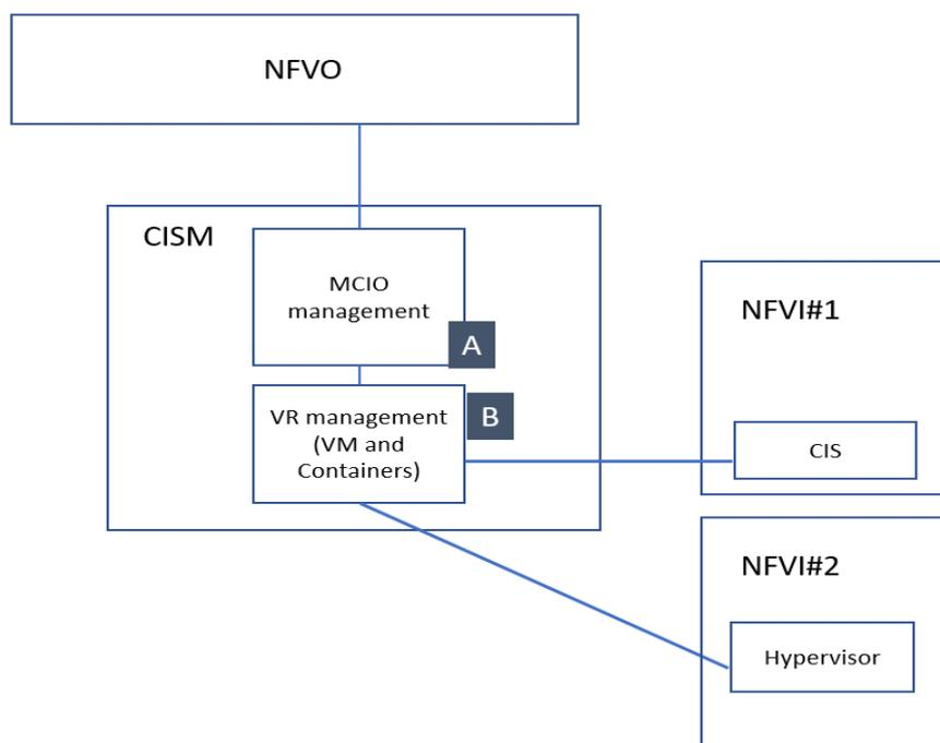
NOTE: The figure focuses on the portion of NFV-MANO architecture relevant for the concepts of architectural impacts.
