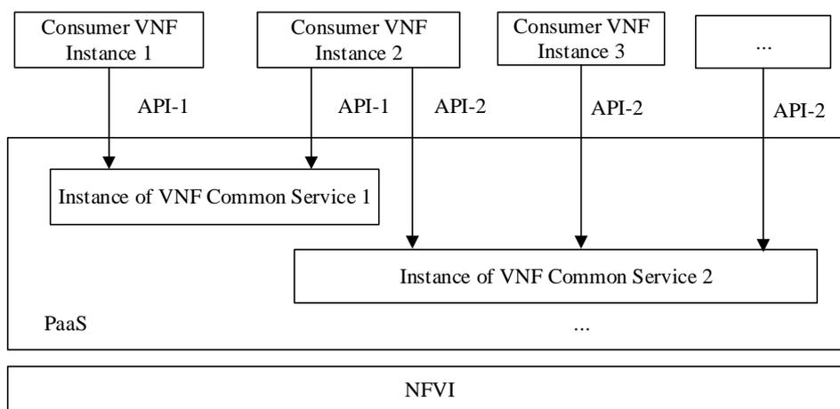
**Figure 5.1.2.1-1: An example to illustrate Consumer VNF instances invoke multiple VNF Common Service instances in PaaS**
