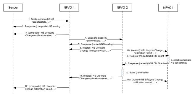
Figure A.1.3b-1: Composite NS scaling in sharing scenario
