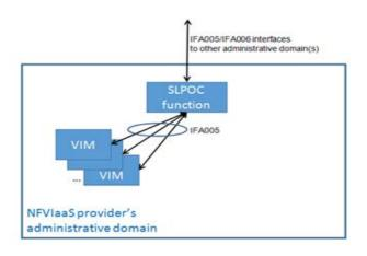
Figure 5.2.5-2: Illustration of SLPOC interfaces
