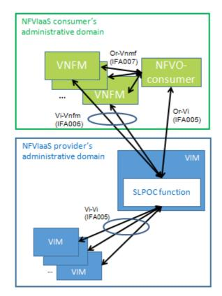
Figure 5.2.7-1: Illustration of SLPOC function integrated into VIM
