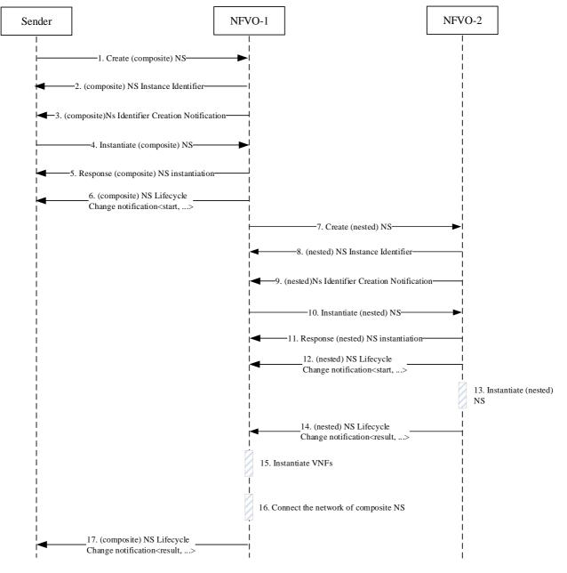
Figure A.1.2a-1: Top-down Composite NS instantiation
