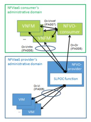
Figure 5.2.7-2: Illustration of SLPOC function integrated into NFVO
