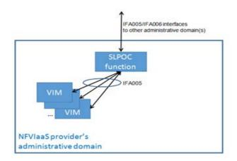
Figure 5.2.4-2: Illustration of SLPOC interfaces
