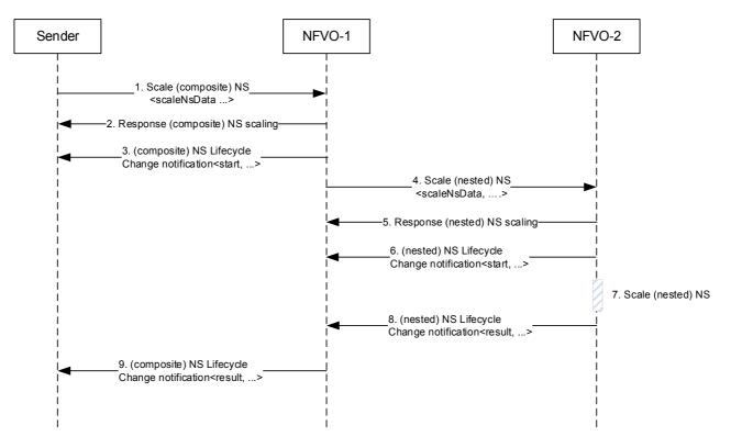
Figure A.1.3a-1: Composite NS scaling
