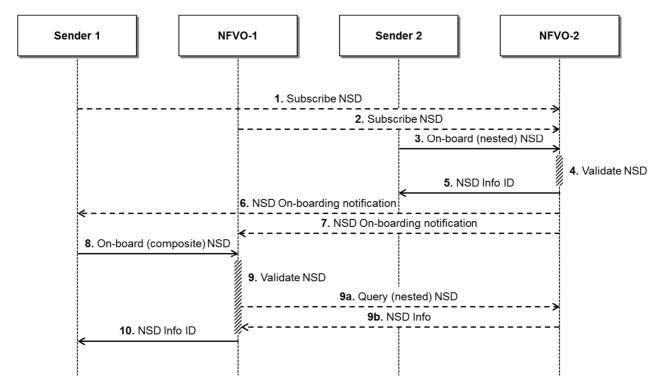
Figure A.1.1-1: Composite NSD on-boarding flow
