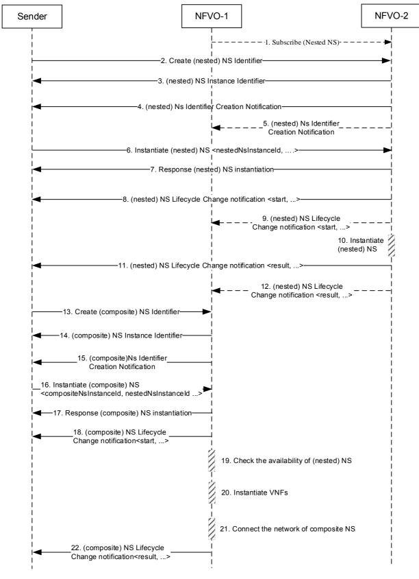
Figure A.1.5-1: Bottom-up Composite NS instantiation
