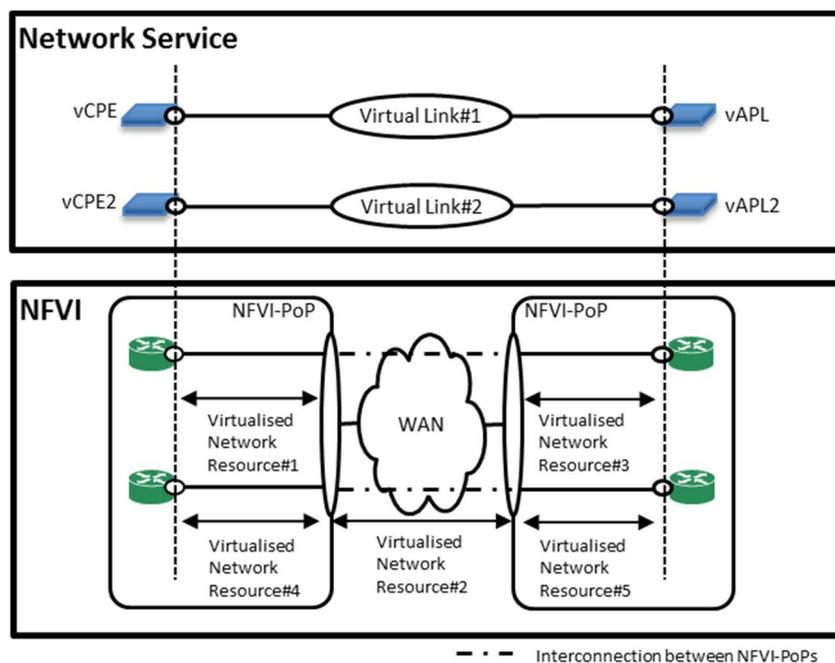
**Figure 5.5.1-1: Connectivity overview for aggregating Virtual Links in the WAN enabling End-to-End Network Service**
