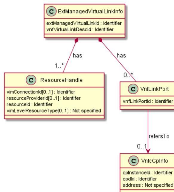
**Figure 6.4.4.2.1-1: Extension to support multiple `ResourceHandle` to realize an `ExtManagedVirtualLinkInfo`**
