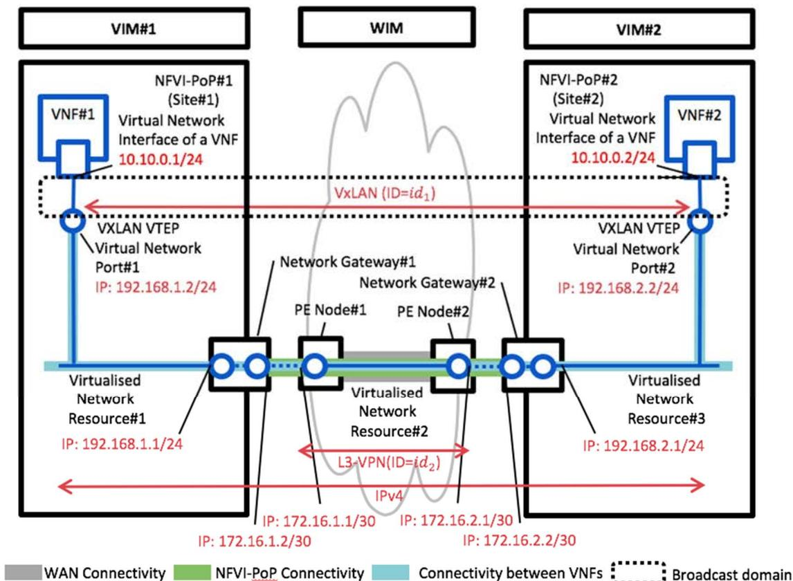
Figure A.3.1.1-1: Overview of VXLAN connection between NFVI-PoPs over L3 WAN connectivity
