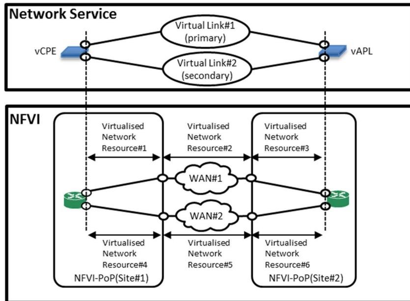
Figure 5.7.1-1: Connectivity overview for multi-site Virtual Link redundancy
