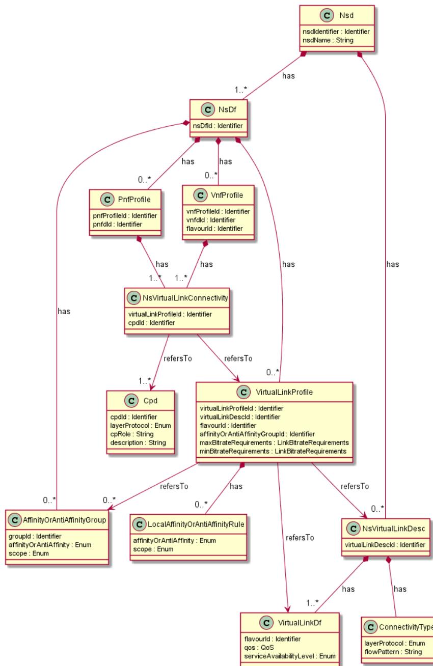
Figure 6.4.2.1-1: Current NSD connectivity model based on ETSI GS NFV-IFA 014 [i.12]
