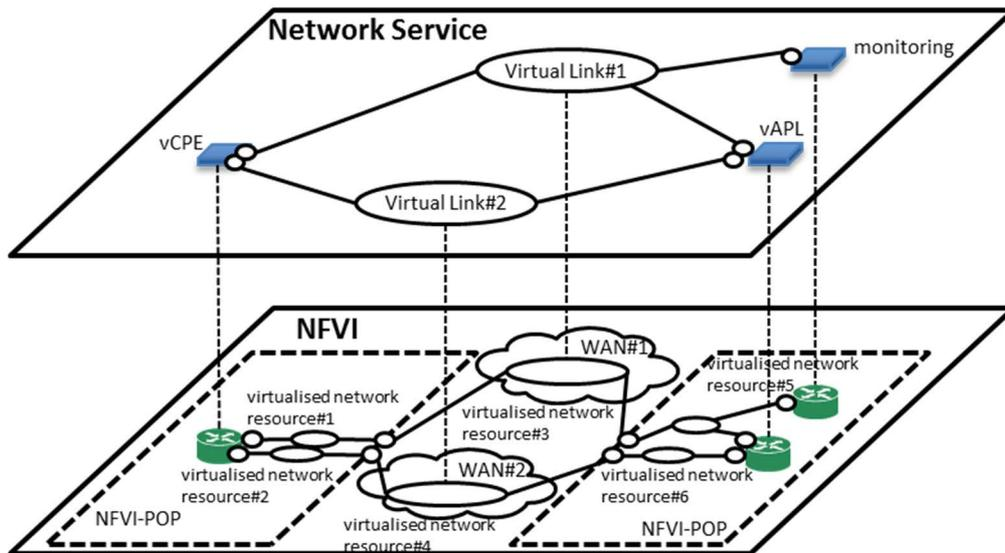
**Figure 5.3.1-1: Connectivity overview for enabling End-to-End Network Service across two WANs**
