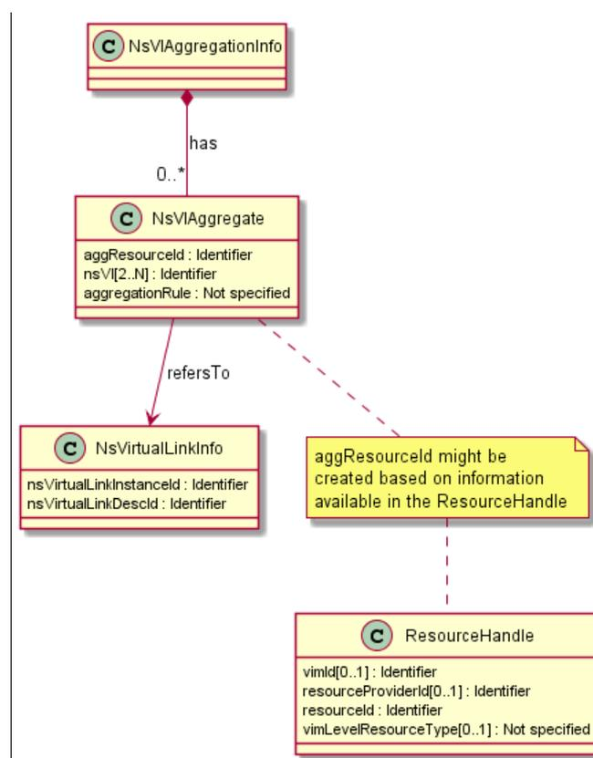
**Figure 6.4.3.2.1-1: Option #1 for NS VL aggregation**
