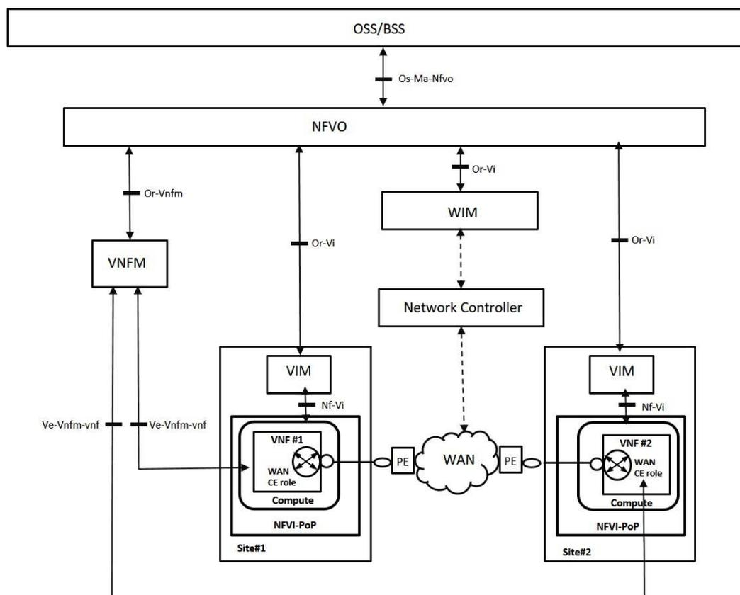
**Figure 5.14.1-2: High level use case of WAN connectivity in compute-only NFVI-PoPs**
