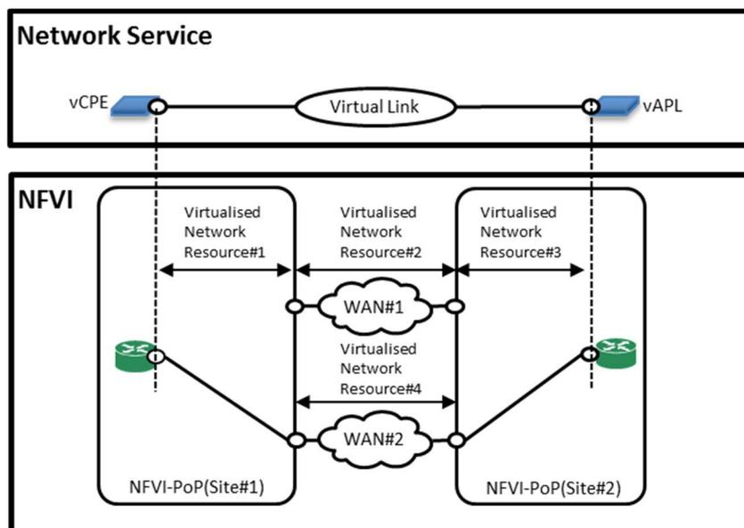
Figure 5.8.1-2: Connectivity overview after multi-site Virtual Link healing
