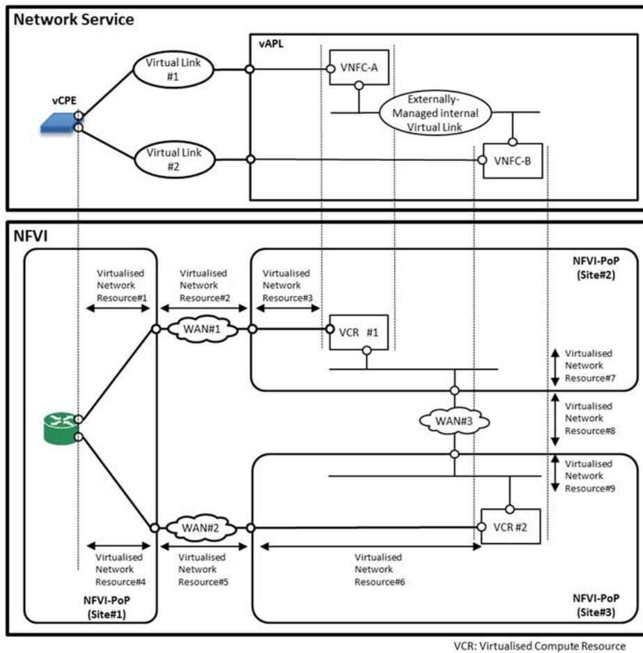
**Figure 5.9.1-1: Connectivity overview for multi-site VNF deployment**
