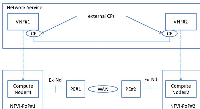
**Figure 5.14.8-1: Direct attachment case between Compute Node and WAN PE**
