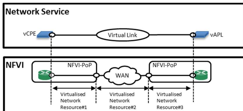
**Figure 5.2.1-1: Connectivity overview for enabling Network Service**
