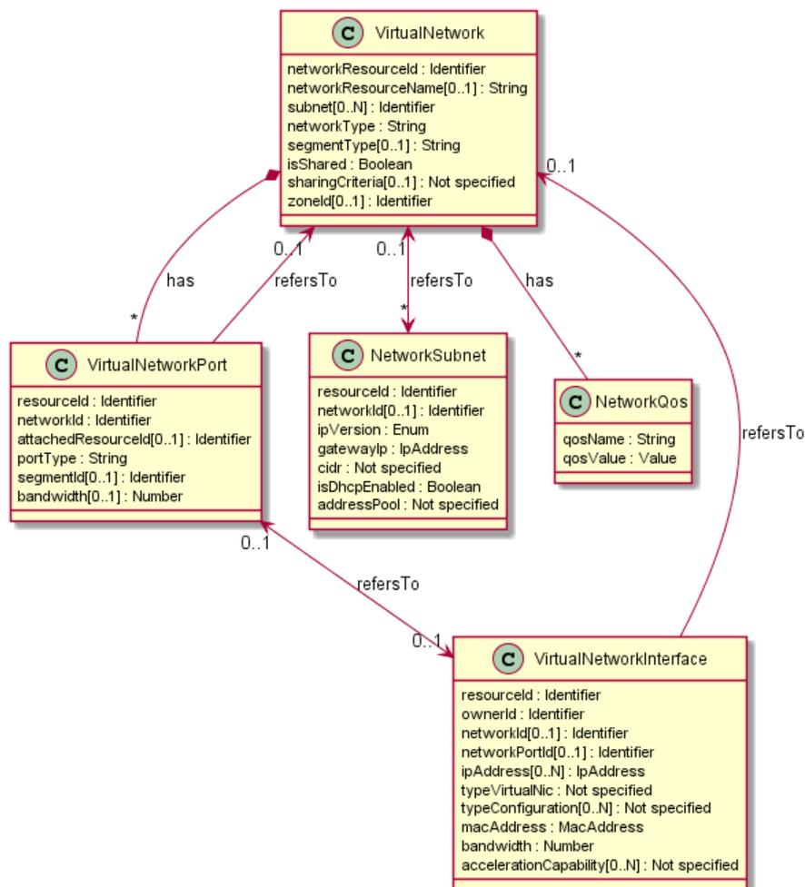
Figure 6.4.5.1-1: Current virtualNetwork information model from ETSI GS NFV-IFA 005 [i.7]
