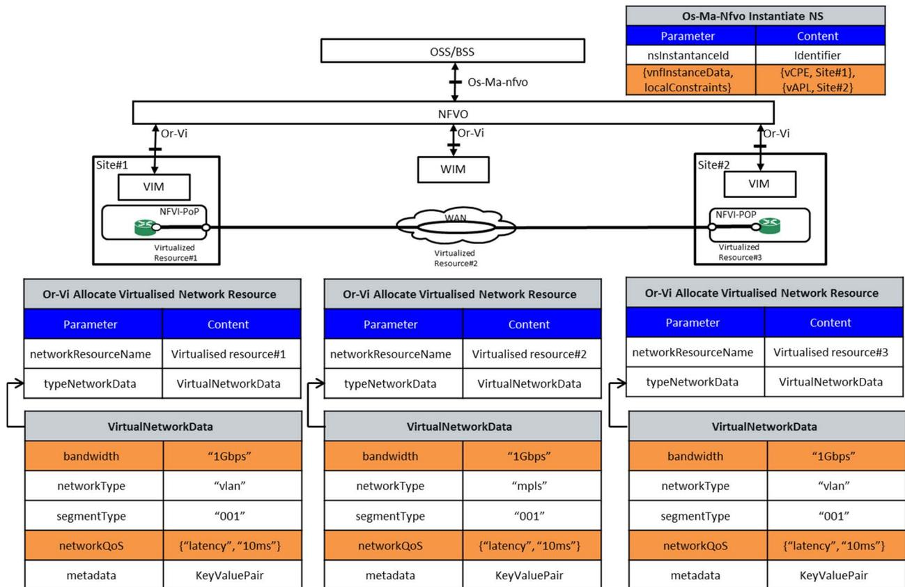
Figure 5.2.7.4-2: Mapping of service instance Model to infrastructure related to an E2E EvCPE service across WAN
