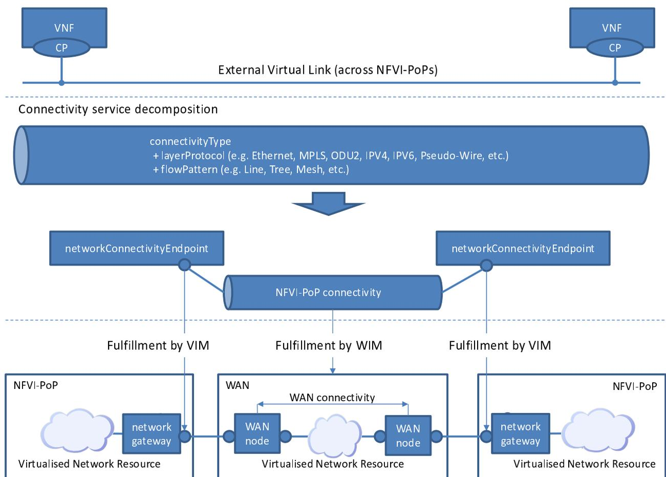
**Figure 6.2.2-1: Mapping and decomposition of connectivity service**
