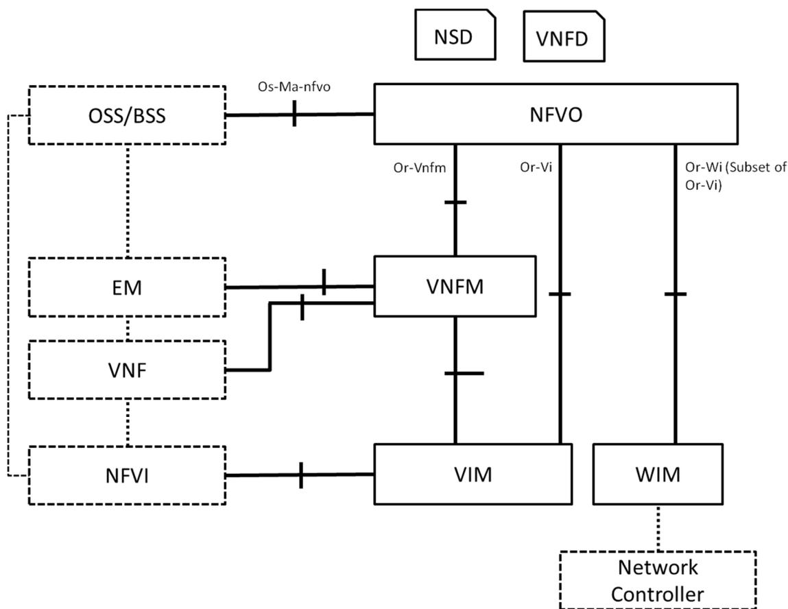
**Figure 6.3.2-1: Managing WIM function blocks using Or-Wi reference point**
