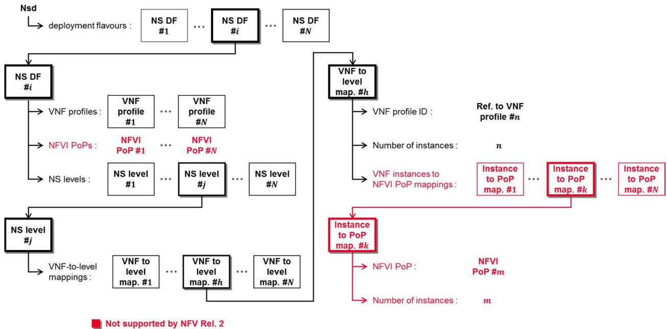
**Figure 5.10.8-3: Potential enhancements directed to IFA 014 aimed at overcoming existing limitations**
