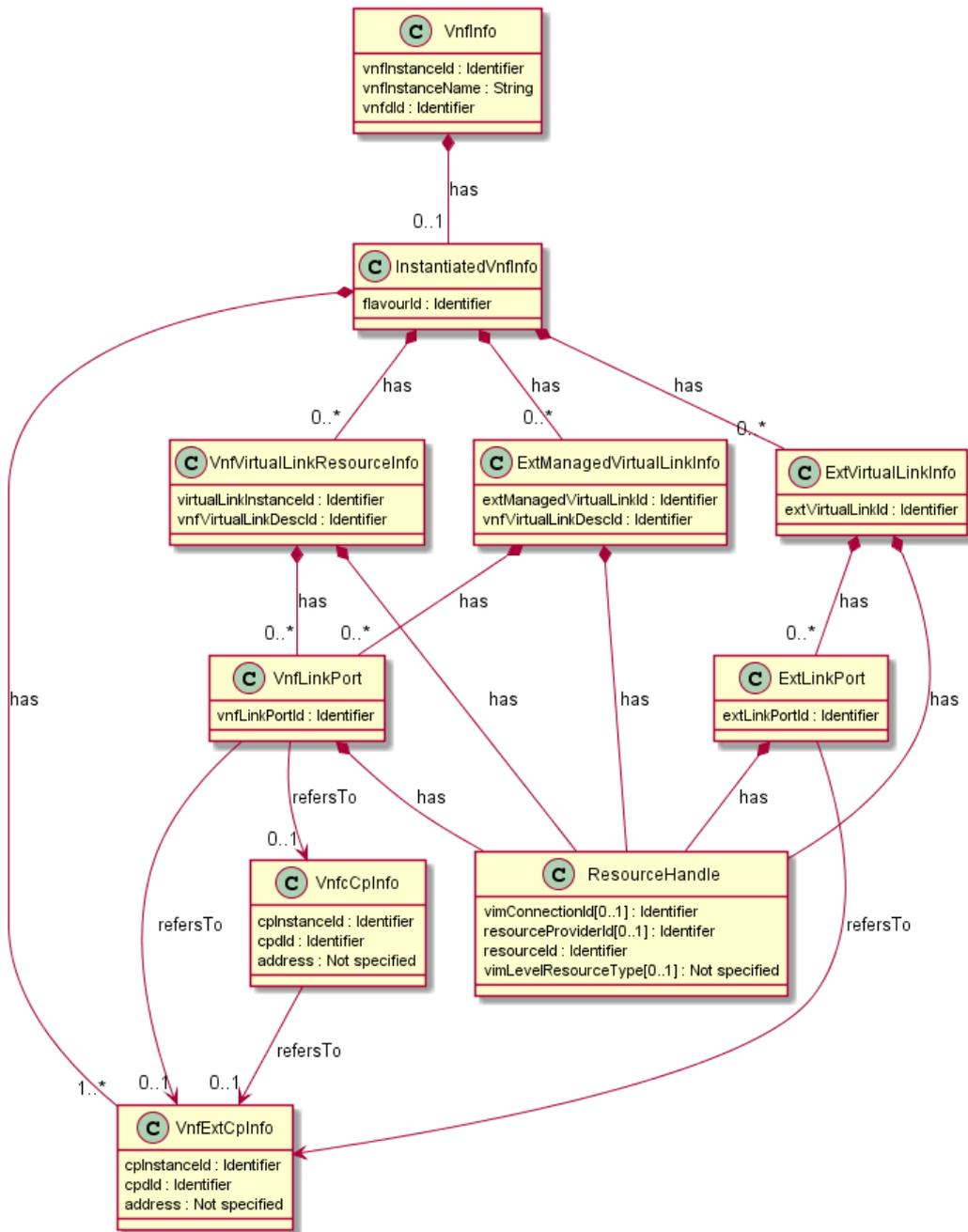
Figure 6.4.4.1-1: Current VNF connectivity information model from ETSI GS NFV-IFA 007 [i.8]
