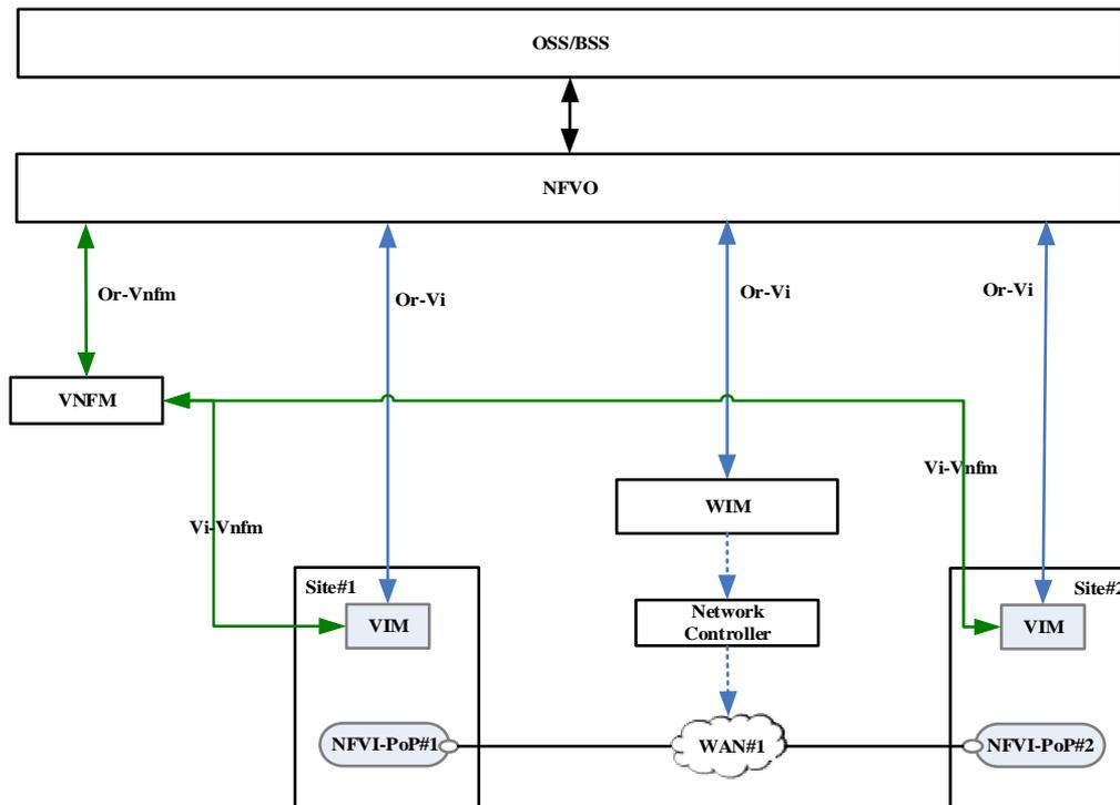
Figure 5.9.1-2: High-level architectural view supporting connectivity for multi-site VNF deployment
