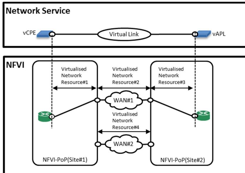
**Figure 5.8.1-1: Connectivity overview for multi-site Virtual Link healing**
