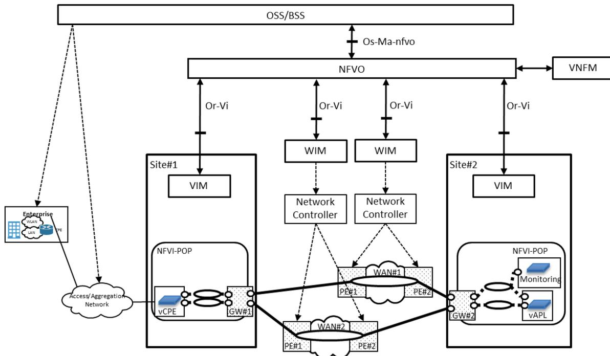
**Figure 5.3.1-2: High-level use case for an E2E EvCPE service across two WANs**
