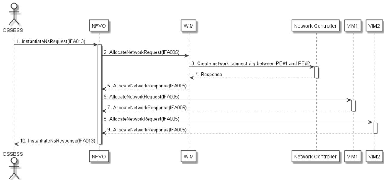
**Figure 5.2.7.4-1: Instantiate a connectivity service**
