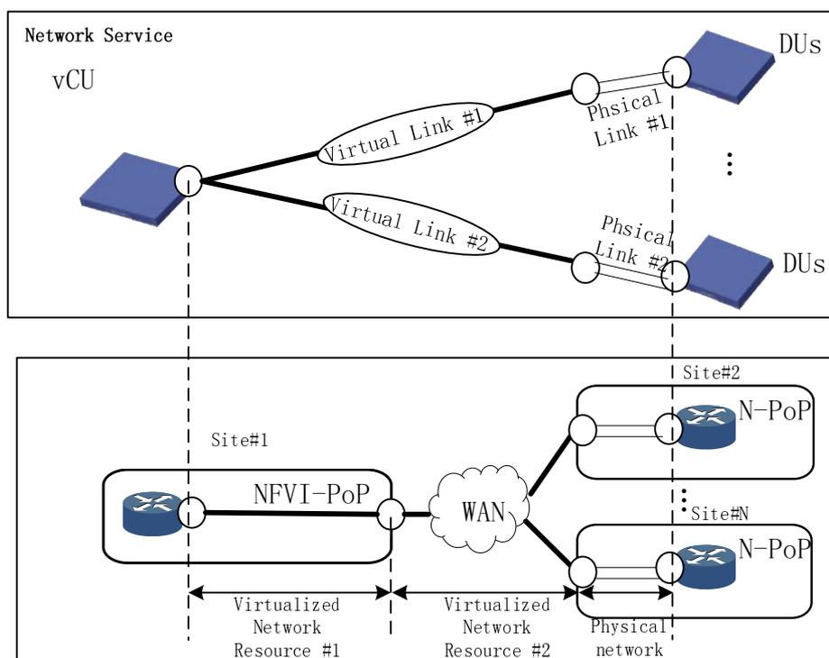
**Figure 5.13.1-1: Connectivity overview for enabling Network Service**
