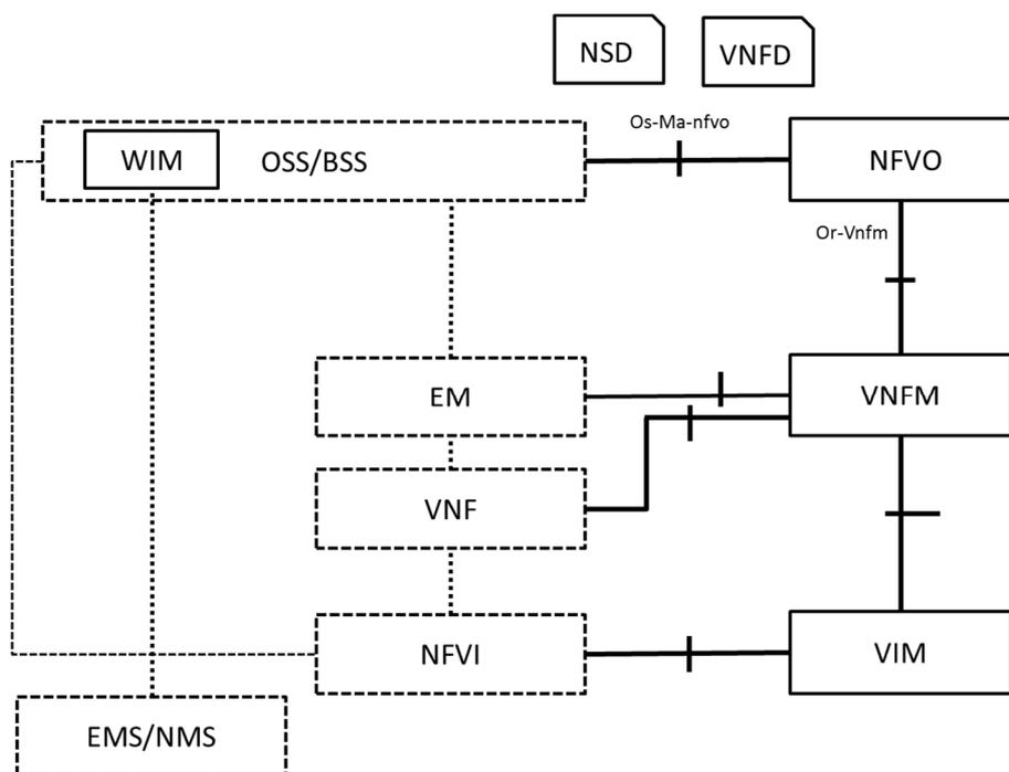
**Figure 6.3.3-1: Managing WIM function blocks using Os-Ma-nfvo reference point**
