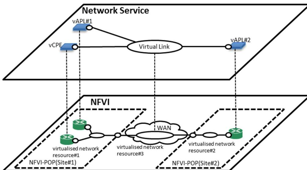
Figure 5.4.1-1: Connectivity overview for enabling NS expansion over WAN
