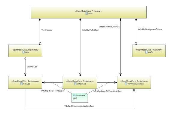
Figure 3: Basic example of a VNF deployment view
