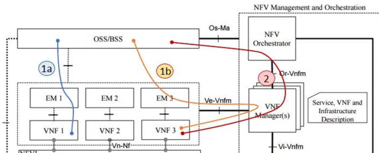
**Figure 5.15.1-1: Alternate configuration paths**
