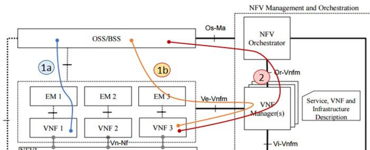
**Figure 5.15.1-1: Alternate configuration paths**
