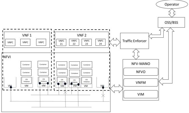
Figure 4.3.3.1-1: Example of relationship between Operator, OSS/BSS, Traffic Enforcer, and NFV-MANO
