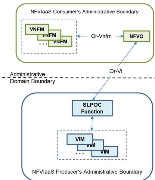
**Figure 5.4.2-5: NFVlaaS-C Management Functions interacting with NFVlaaS-P's VIM(s) via SLPOC in indirect mode**
