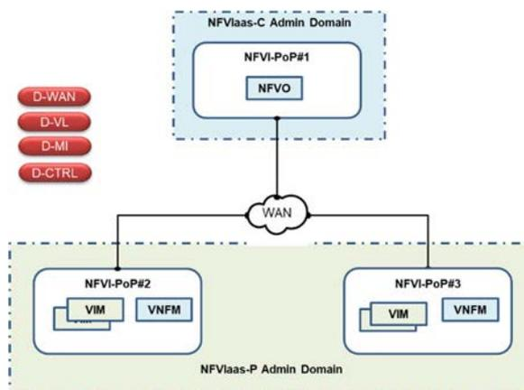
**Figure 5.4.4-2: NFV-MANO deployment in multi-site environment with the NFVaaS-C's NFV-MANO functions distributed in different NFVI-PoPs**
