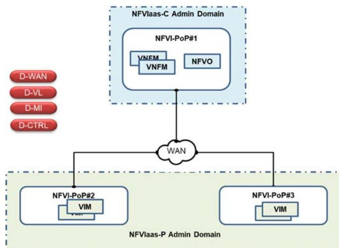
**Figure 5.4.4-1: NFV-MANO deployment in multi-site environment with the NFVaaS-C's NFV-MANO functions located in the same NFVI-PoP**
