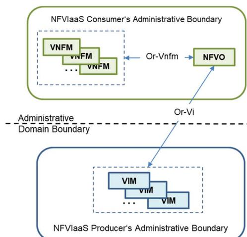
**Figure 5.4.2-3: NFVlaaS-C Management Functions interacting with NFVlaaS-P's VIM(s) via MLPOC in indirect mode**
