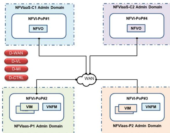
**Figure 5.4.4-4: NFV-MANO deployment in multi-site environment with different NFVlaaS-Cs managing a composite NS deployed across different NFVlaaS-P's administrative domains**
