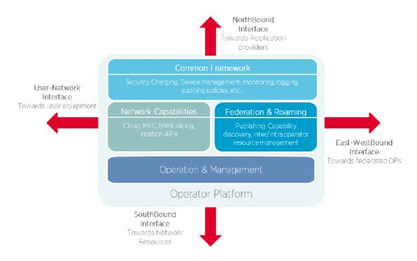
Figure 4.2-1: High level GSMA Operator Platform building blocks (source: [i.4])
