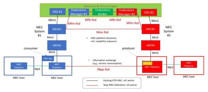
Figure 6.5.2-6: All proposed MEC federation reference points assuming the existence of a Federation Broker communicating with multiple Federation Managers
