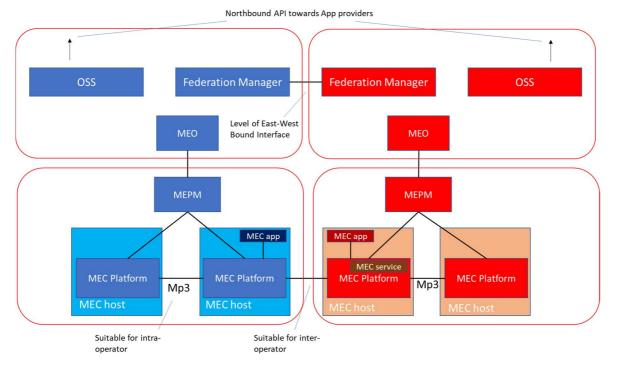
Figure 6.1.2-1: The considered hierarchical functional levels based on which a MEC federation can be formed by means of a proper signalling
