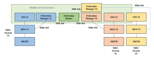
NOTE: In this implementation variant, a single Federation Broker for the whole MEC federation is considered.
