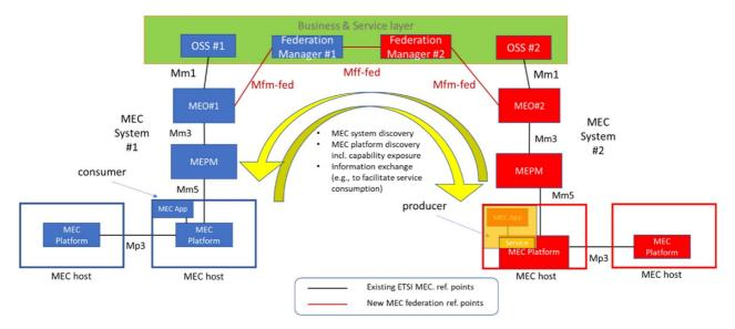
Figure 6.5.3-2: Conceptual diagram with all proposed MEC federation reference points assuming a Federation Manager per MEC system
