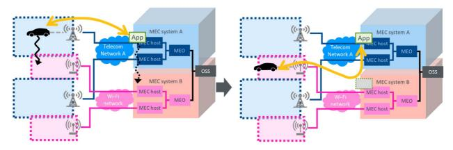
Figure 5.4.1-4: Abstract level of behaviour in case of MEC service remote consumption
