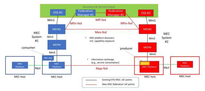
Figure 6.5.2-4: All proposed MEC federation reference points assuming a Federation Manager per MEC system
