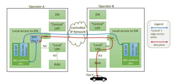
Figure 5.8.1-1: Scenario of edge node sharing (source: 5GAA)
