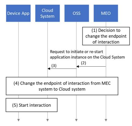
Figure 6.6.2-1: High-level information flow of sending request to instantiate or re-start the application instance via OSS
