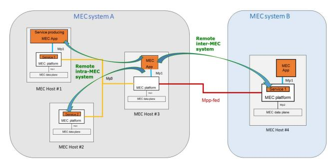
Figure 6.5.2-1: MEC federation scenario enabling edge service consumption across MEC systems
