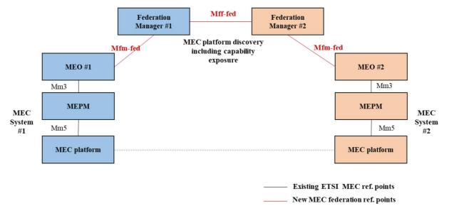
Figure 6.4.3-1: Inter-MEC platform discovery by using the Federation Manager modules
