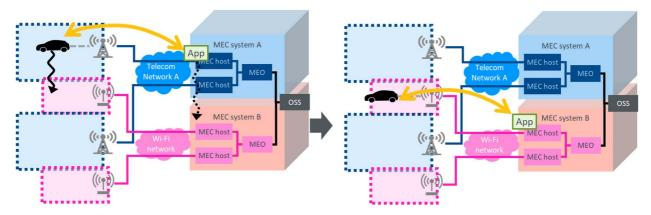
Figure 5.4.1-1: Abstract level of behaviour in case of two MEC systems in one MNO environment
