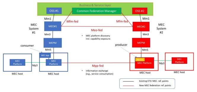
Figure 6.5.2-5: All proposed MEC federation reference points assuming a single Federation Manager, the scope of which is the whole MEC federation
