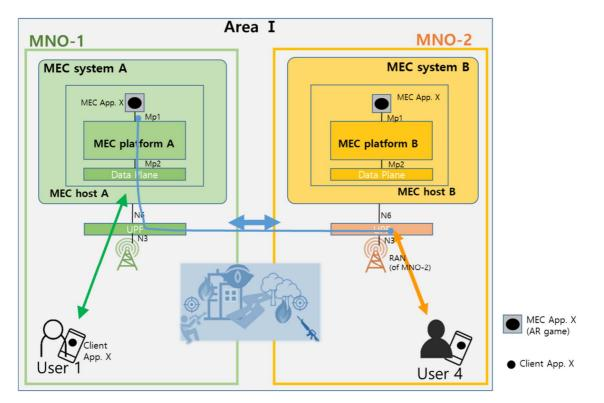
NOTE: In this environment, users of different MNOs, user 1 of MNO-1 and user 4 of MNO-2 can join a multiplayer interactive AR game and play together. The MEC platform B switches the traffic from user 4 for MEC application X to MEC platform A.
